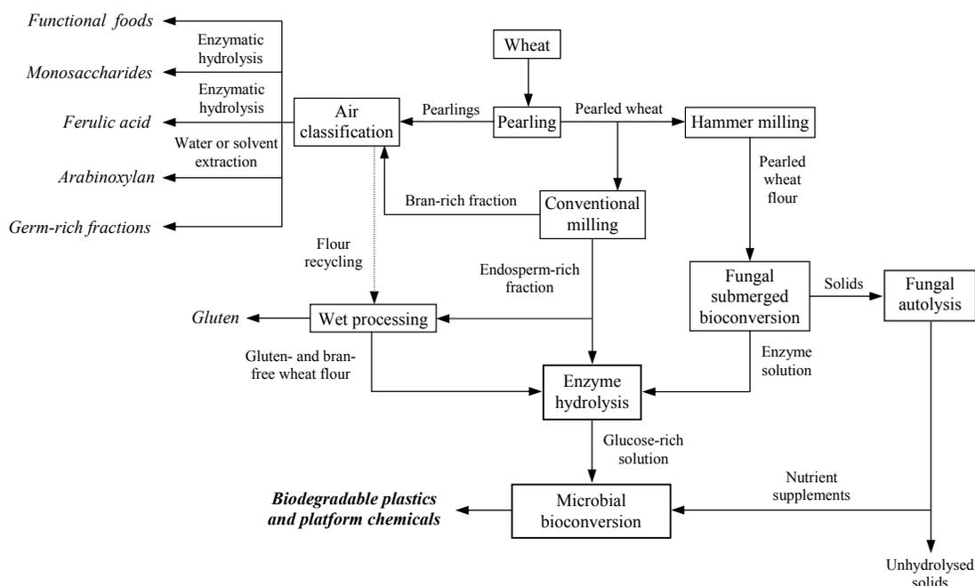
**Figure 1** Proposed wheat-based biorefinery for the production of PHB and succinic acid
