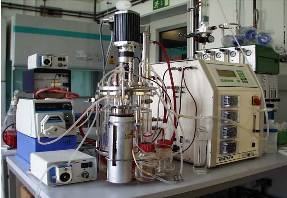
Figure 1: Setup of the fixed-bed reactor system showing the fixed bed reactor in the middle in front of the double walled conditioning vessel. On the right hand side the control unit equipped with four peristaltic pumps for taking samples can be seen. On the left side the circuit pump is placed in the back. The peristaltic pump in the front was used for batch harvesting. Feed and harvest vessels are shown next to the fixed bed.
