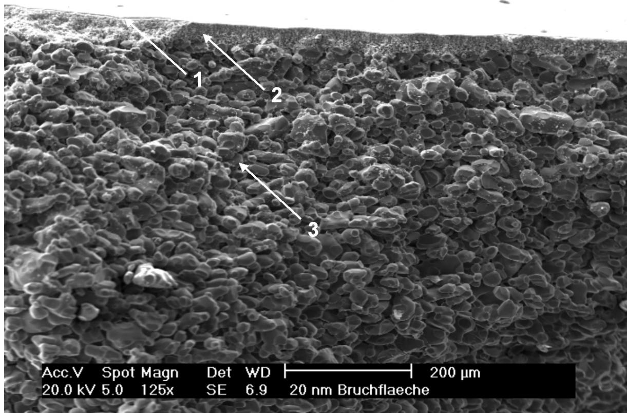
Figure 3: Cross section of a ceramic membrane showing three different layers. The one at the bottom is the support layer (3), in the middle (2) is a layer with a smaller core diameter and on the top (1) the functional membrane surface that is responsible for the membrane separation properties.
