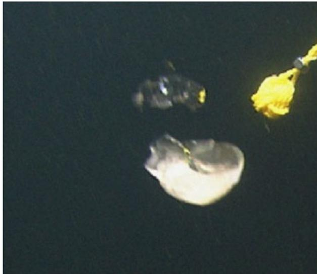
**Fig. 3.** CO<sub>2</sub> Drop Descending after Released at 500m Depth
