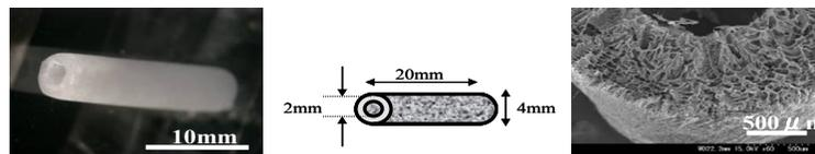
Figure 1. Porous tubular scaffold made of PLLA
