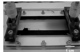
**Figure 1.** A flat-plate bioreactor.
