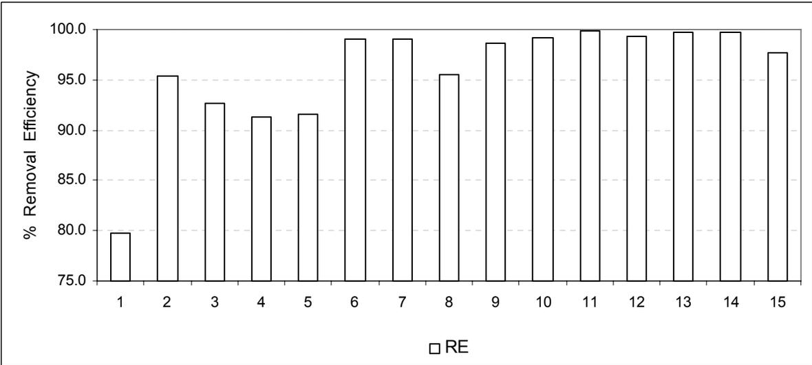
Figure 5. The removal efficiency of salt from frozen synthetic seawater using the chiller reactor at ICES.
