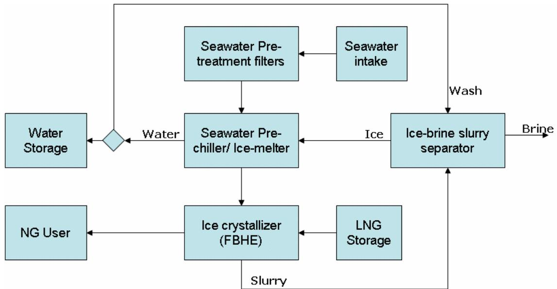
Figure 1. A schematic concept of the process envisioned for saltwater freezing using enthalpy from LNG regasification.
