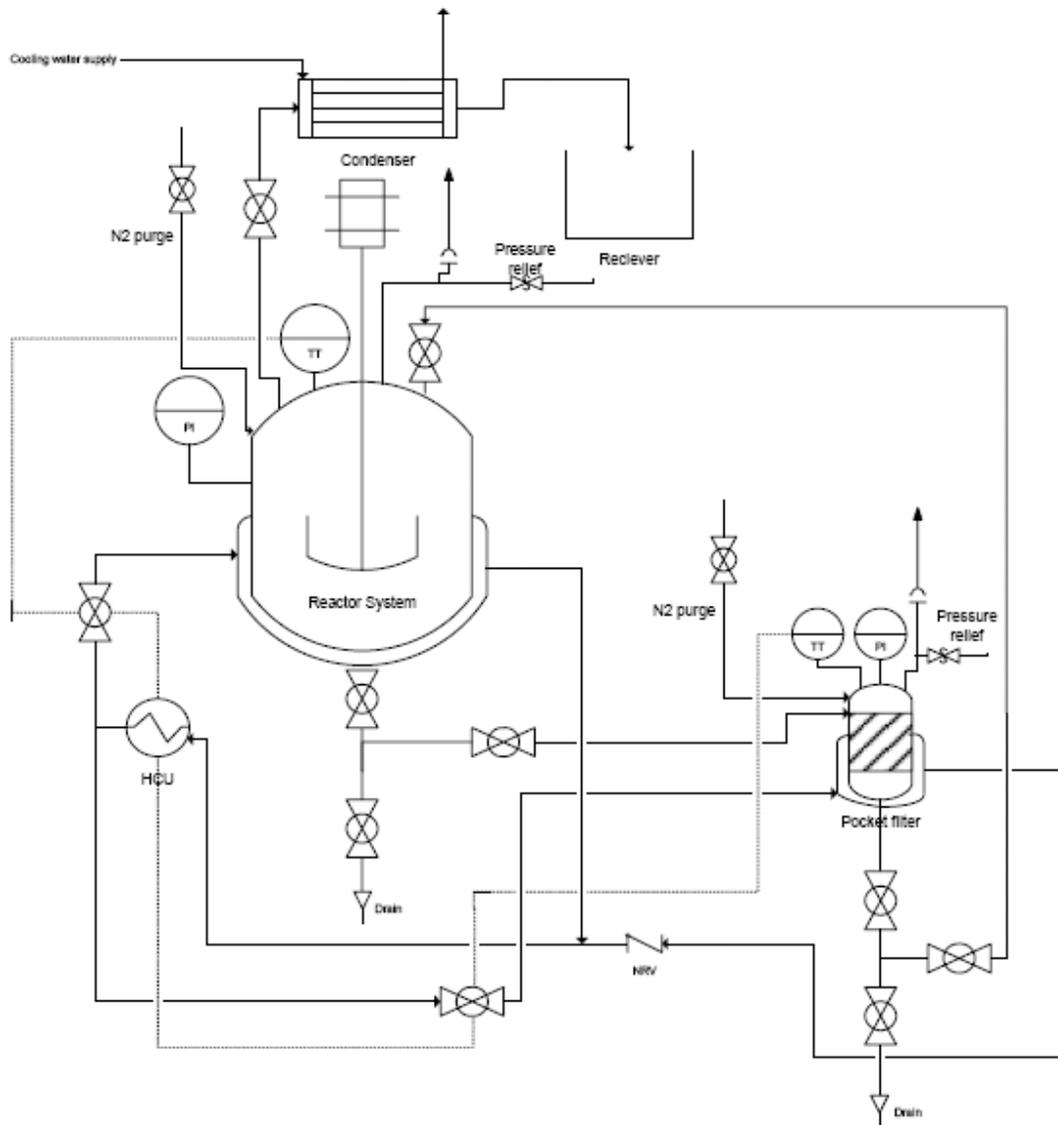
Figure 3. Batch reactor and filter setup. The filter is not utilized in the experiments.
