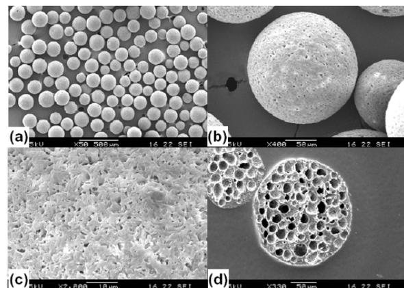
Figure 1. (a) and (b) SEM images of PHBV microspheres illustrating their spherical shape and uniform size; (c) magnified image of (b) showing a rough surface with nano-pores; (d) cross-section of the microsphere;
