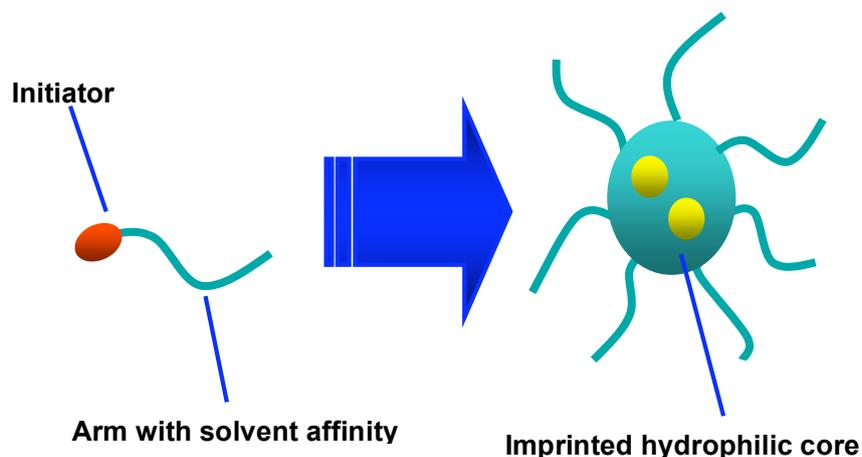
**Fig.1:** Molecularly imprinted star polymer (StarMIP)
