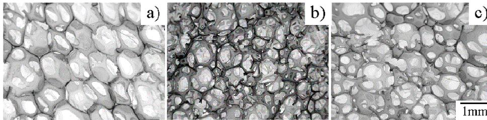
**Figure 3.** SEM images: (a) control;(b) 30% SAN; and (c) 30% SBOP
