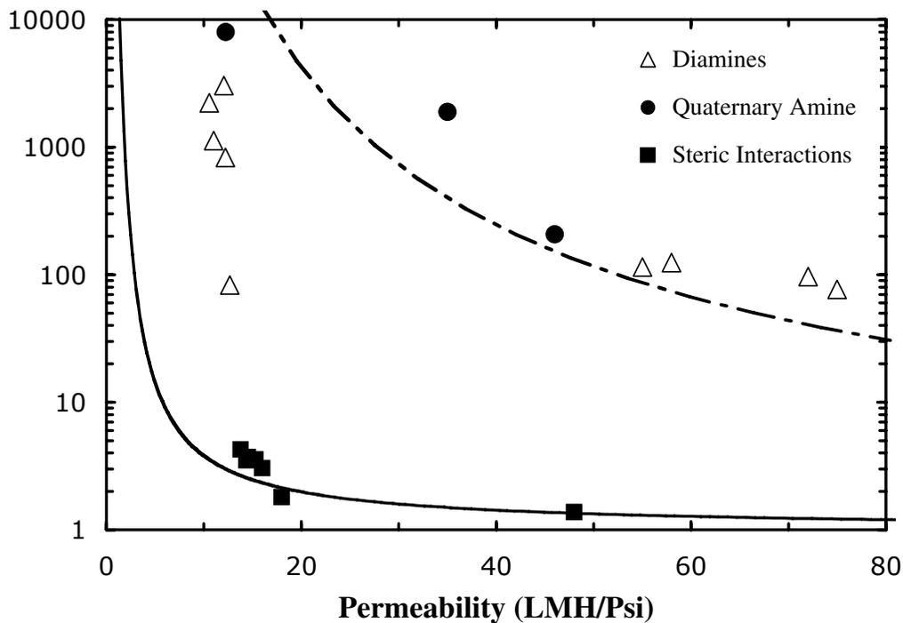
**Figure 3:** Permeability-Selectivity analysis for membranes developed using different surface modification chemistries. The solid curve represents the predicted trade-off between the permeability and selectivity for cytochrome c through an uncharged membrane while the dashed curve represents the predicted trade-off for membranes with a charge density of  $5.5 \times 10^{-3} \text{ C/m}^2$ .
