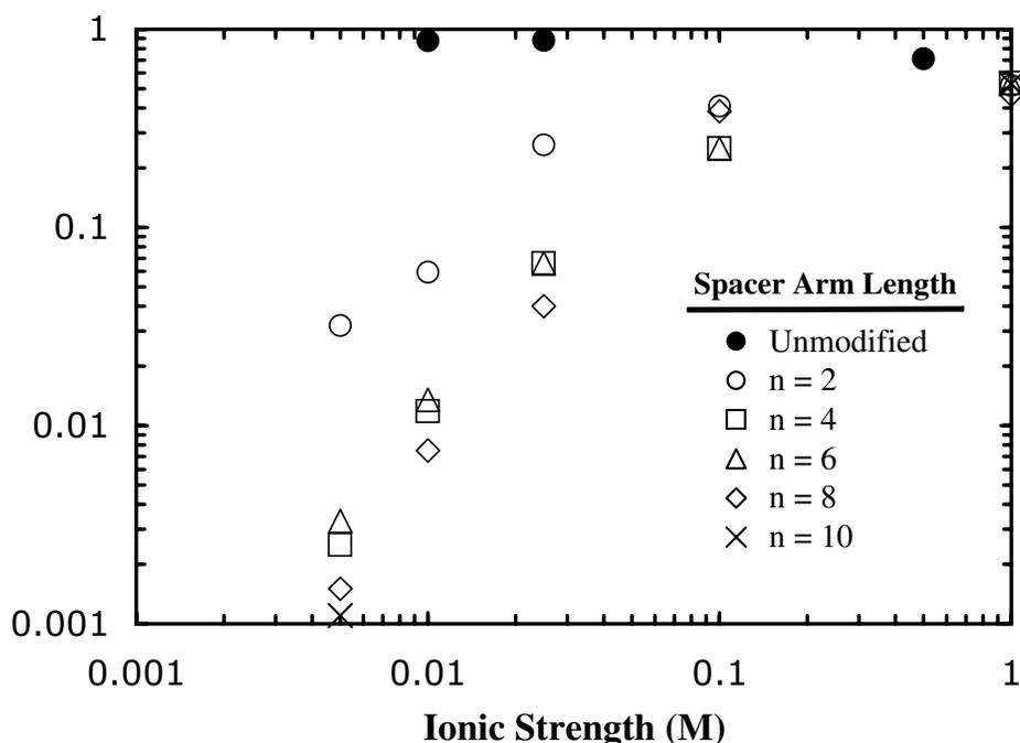
**Figure 2:** Observed sieving coefficients for cytochrome c as a function of solution ionic strength through a series of charge-modified CRC 30 kD membranes possessing different spacer arms
