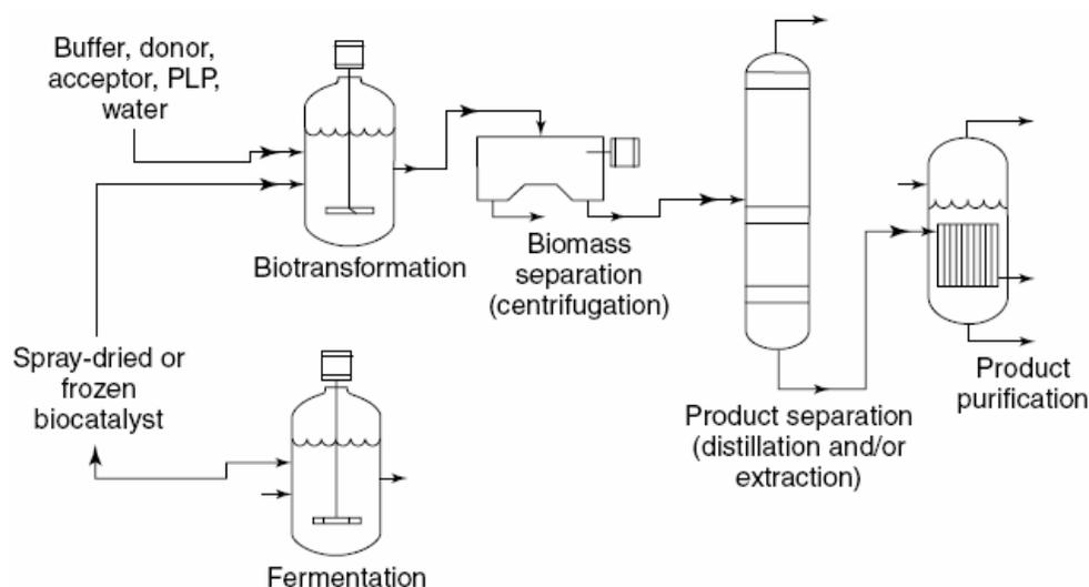
Figure 2: Biotransformation process for production of substituted (S)-aminotetralins (viii).
