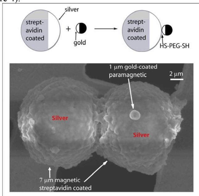
**Figure 4.** SEM image of (right) a 7- $\mu\text{m}$  and a 1- $\mu\text{m}$  magnetic particle. The orientation of the particles (top) suggests that the smaller particle is specifically bound to the larger particle by polymer cross-bridges.
