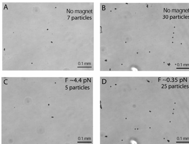
**Figure 6.** Images of streptavidin-coated magnetic particles interacting with biotinylated membranes on a microscope slide in the absence or presence of an external magnetic field. (A) & (B) No magnetic field, (C) 4.4 pN and (D) 0.35 pN.
