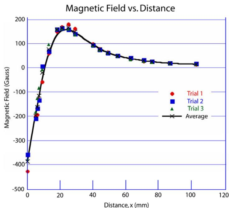
**Figure 2.** Magnetic field of the permanent ring magnet as a function of distance, x (mm), away from the surface.
