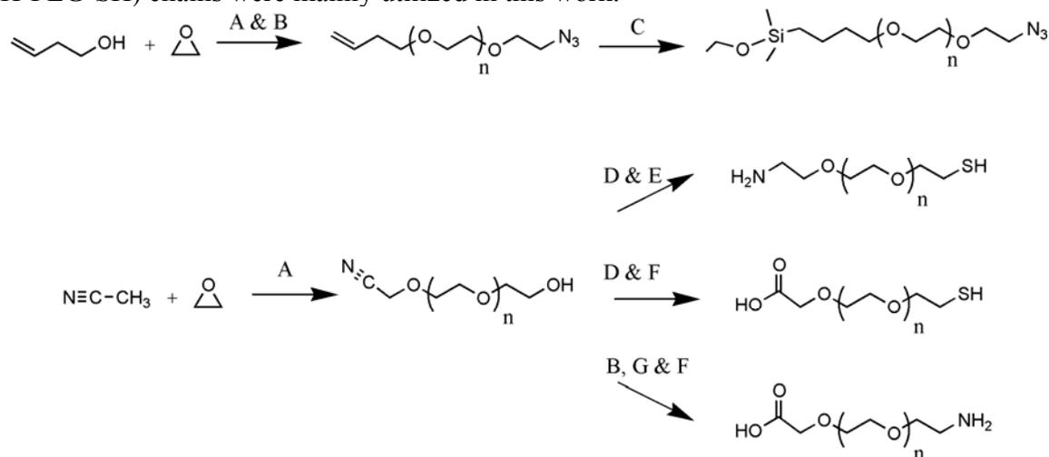
**Figure 1.** Synthetic route for the preparation of PEG linkers. Conditions: A) K / Naphthalenide; B) MsCl, Et<sub>3</sub>N then NaN<sub>3</sub>; C) HSi(CH<sub>3</sub>)<sub>2</sub>OEt, [Pt]; D) MsCl, Et<sub>3</sub>N then CH<sub>3</sub>COSH; E) LiAlH<sub>4</sub>, THF; F) HCl, H<sub>2</sub>O,  $\Delta$ ; G) PPh<sub>3</sub>, H<sub>3</sub>PO<sub>4</sub>.<sup>19</sup>
