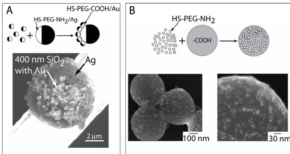
**Figure 3.** (A) SEM image of “half-raspberries” assembly of two complimentary-functionalized SiO<sub>2</sub> particles. (B) SEM image of “whole-raspberries” assembly of complimentary-functionalized Au nanoparticles and polystyrene particles.<sup>19</sup>
