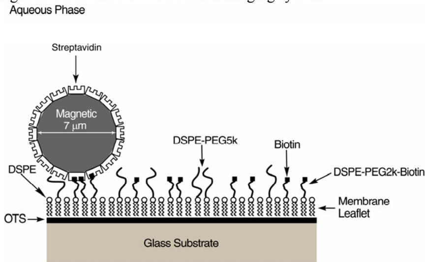
**Figure 5.** Schematic drawing to illustrate the interaction between the streptavidin-coated magnetic particles and the biotinylated model membrane surfaces in Figure 6.
