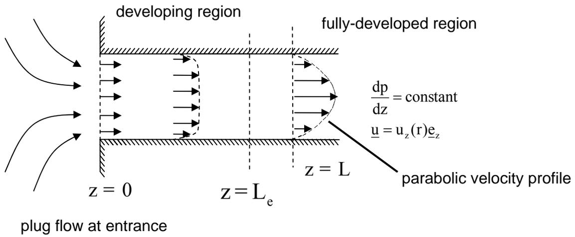
**Figure 1. Schematic of Entry Length Problem**
