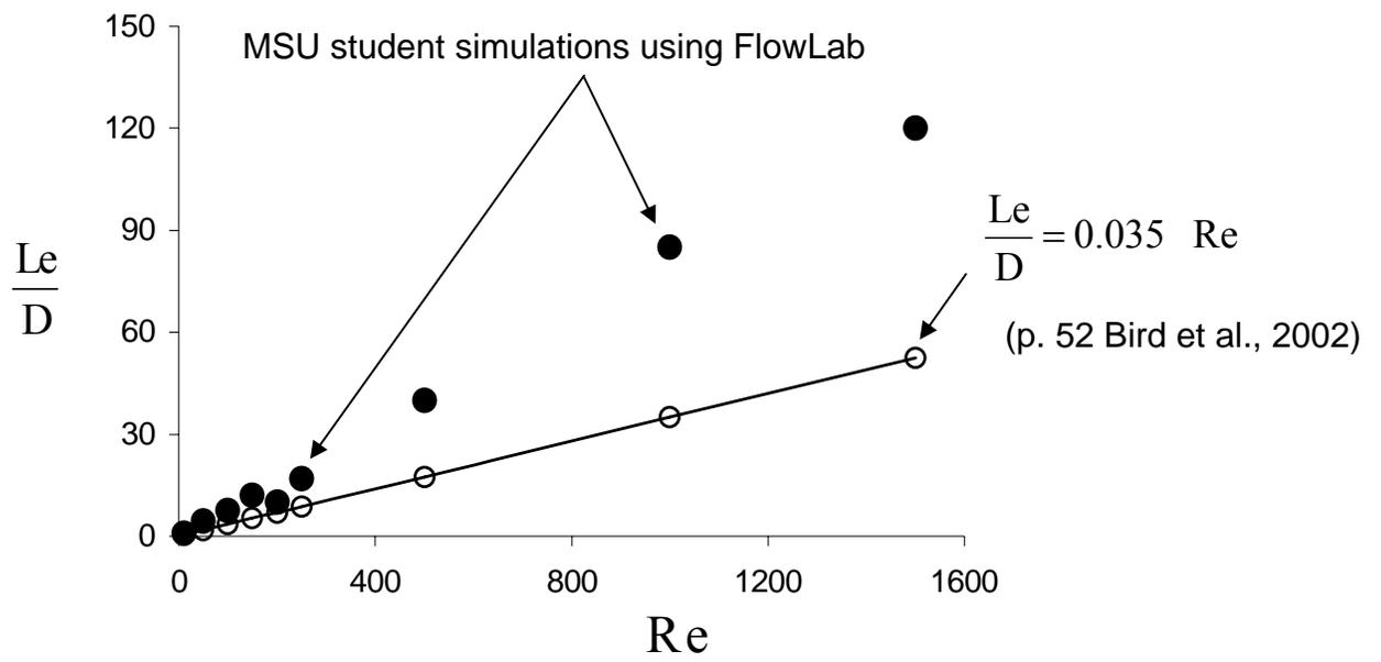
**Figure 3. Entrance length for fully-developed pipe flow**
