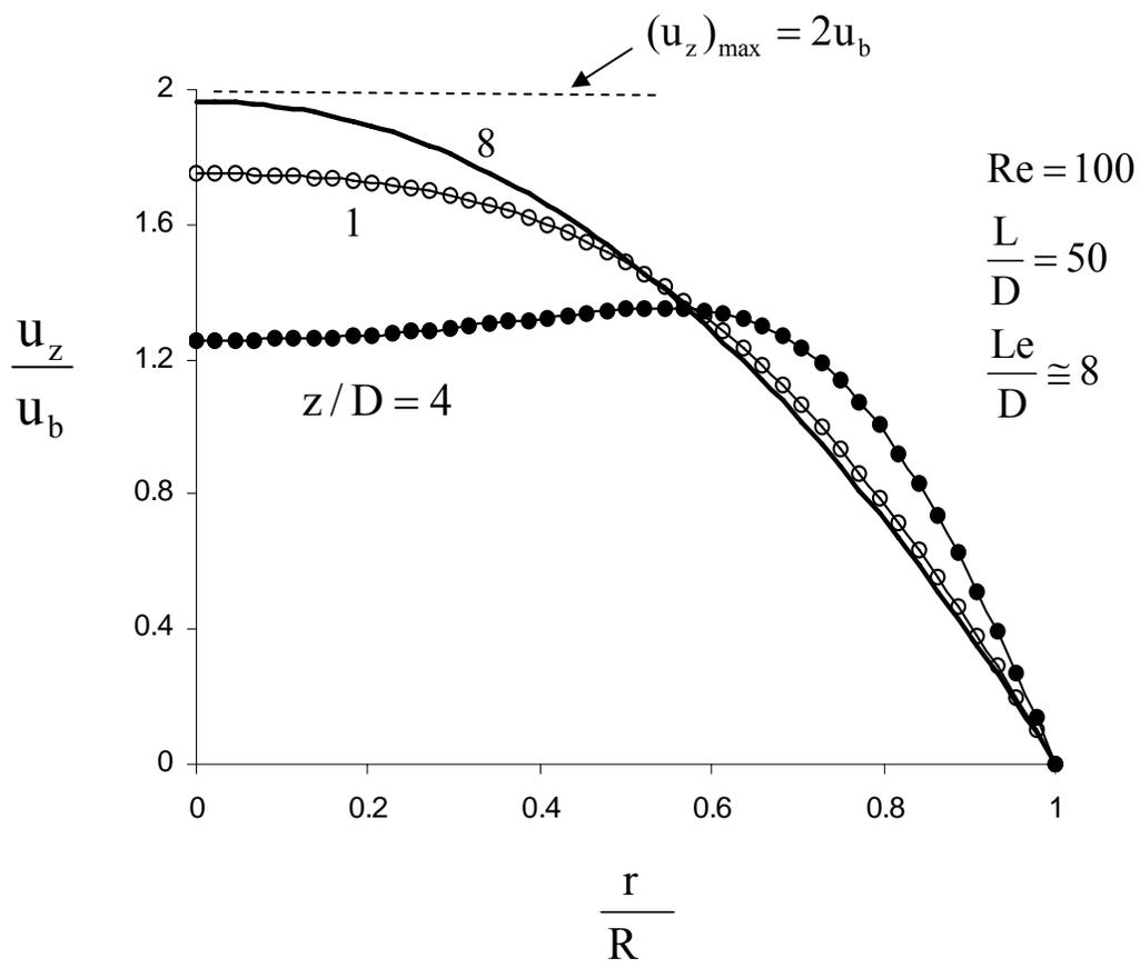
**Figure 2. Developing Axial Velocity Profiles**
