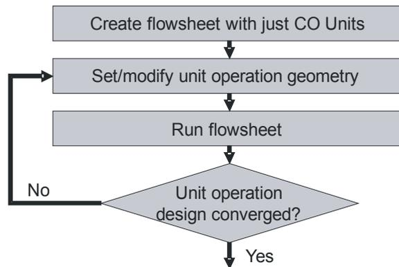
**Figure 4. Simulator as interface**
