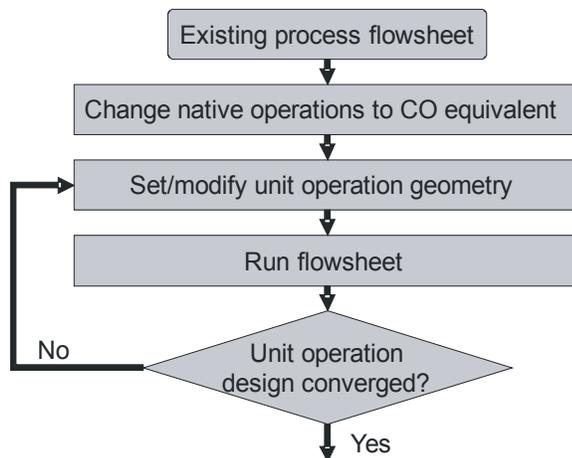
**Figure 2. Embedded simulation**
