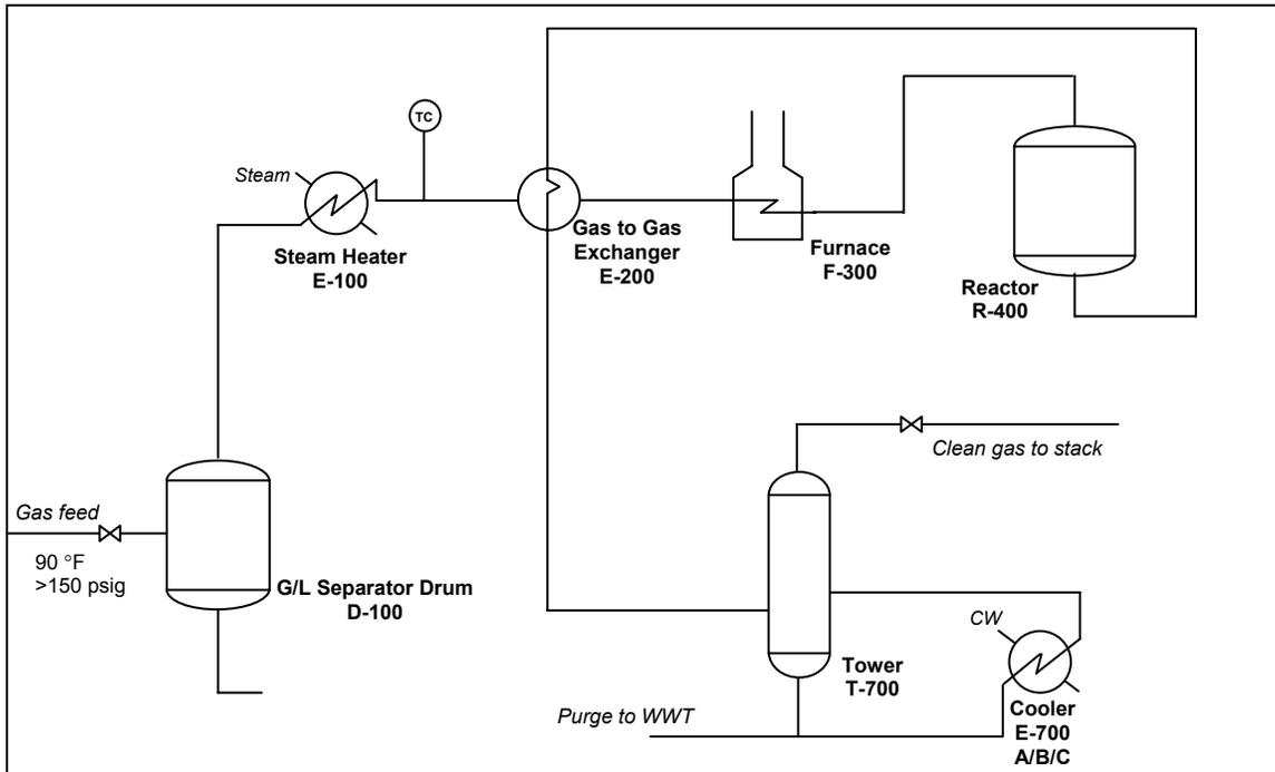
**Figure 1. Gas processing flow sheet**
