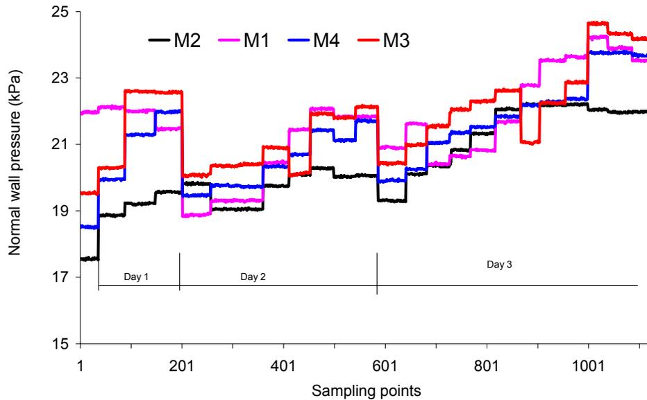
Figure 3. The development of pressures on transducers (the data in each step was obtained in two minutes measurement, each step with a two-hour interval)
