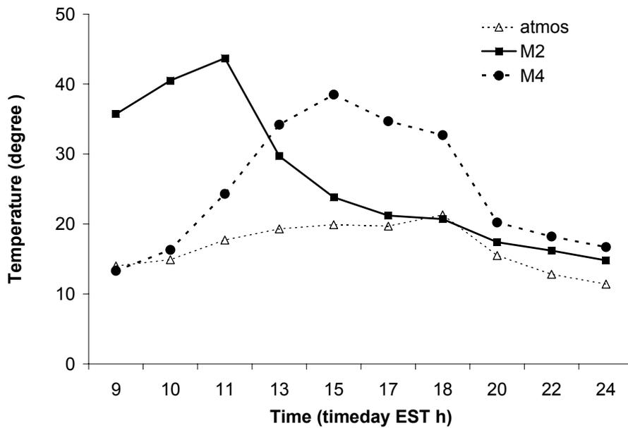
Figure 2 Variation of temperature on the walls along generators M2, M4 in response to the ambient temp. (M2 diametrical opposite to M4).
