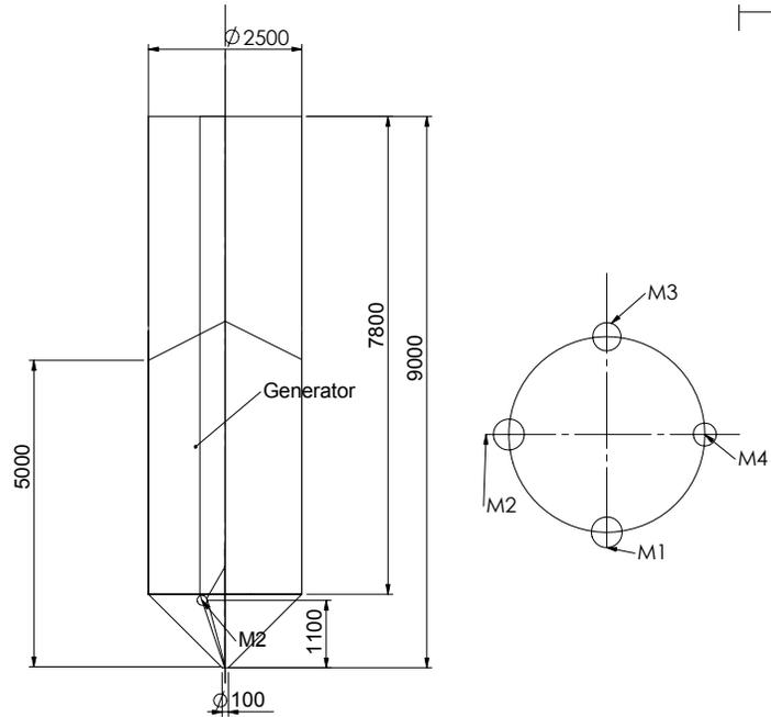
Figure 1. A full scale axi-symmetrical silo, and locations of pressure transducers
