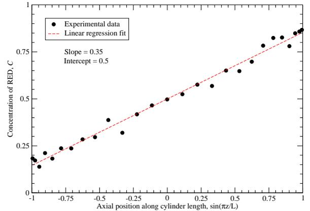
Figure 2: Fraction of red particles plotted against the entire length of the cylinder
