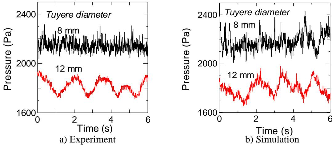
Fig. 4 Pressure fluctuations in the raceway
