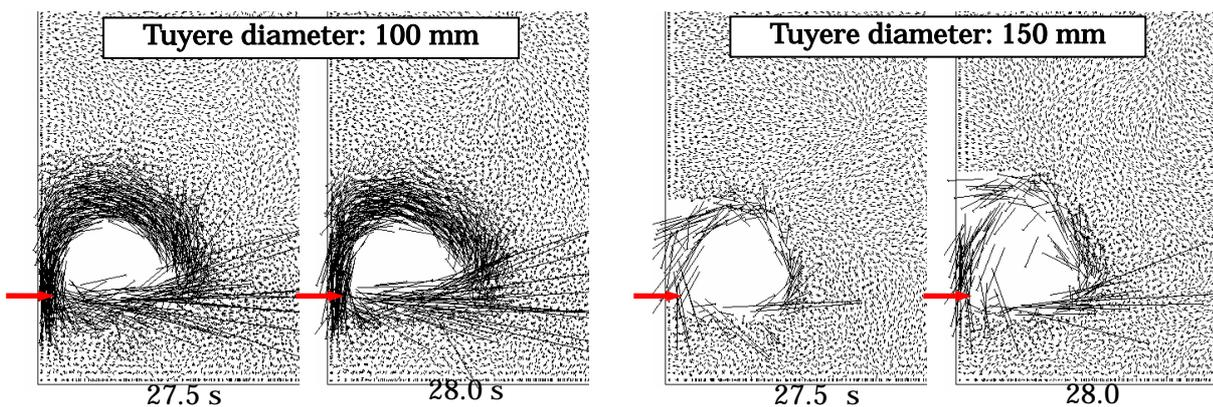
Fig. 6 Effect of tuyere diameter on raceway stability ( $V_b=2.2 \text{ m}^3/\text{s}$ )
