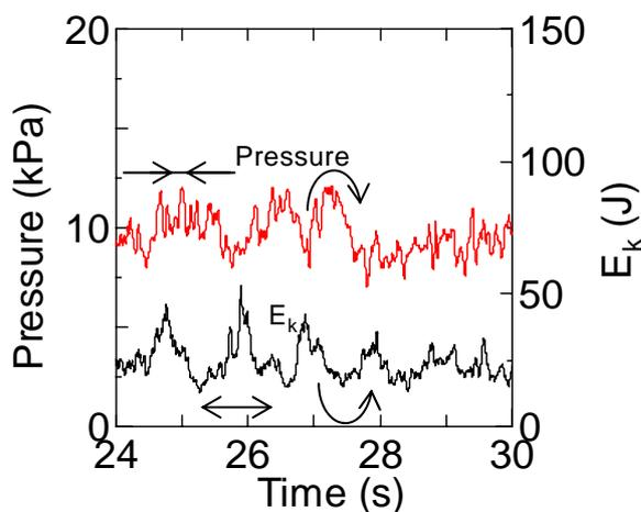
Fig. 7 Fluctuations of the pressure and kinetic energy with unstable raceway ( $V_b=2.2 \text{ Nm}^3/\text{s}$ ,  $D_{ty}=150 \text{ mm}$ )
