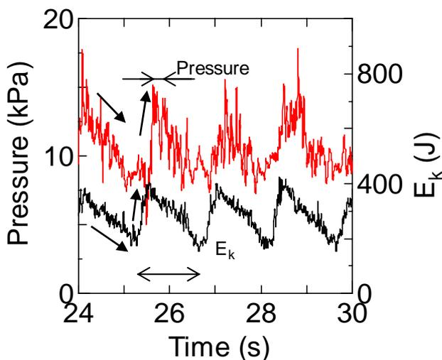
Fig. 9 Fluctuations of pressure and kinetic energy with unstable raceway ( $V_b=2.6$   $\text{Nm}^3/\text{s}$ ,  $D_{ty}=100$  mm)
