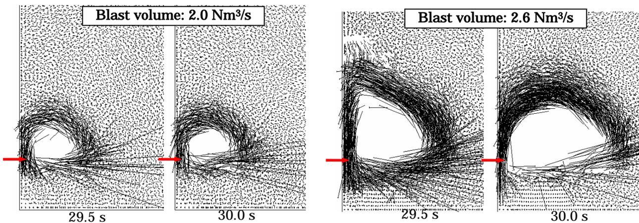
Fig. 8 Effect of blast volume on raceway stability (Velocity vectors of particles,  $D_t=100$  mm)
