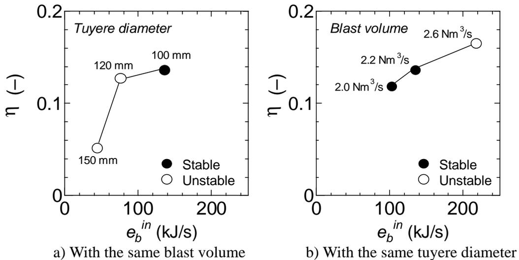
**Fig. 10** Effect of blast energy on the efficiency of the energy transfer from gas to particles
