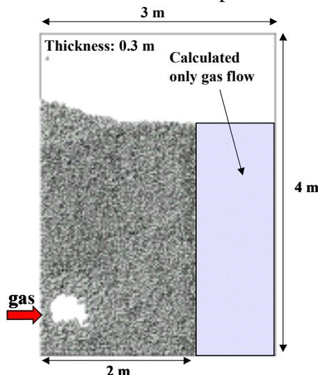
Fig. 5 Geometries used in Simulation
