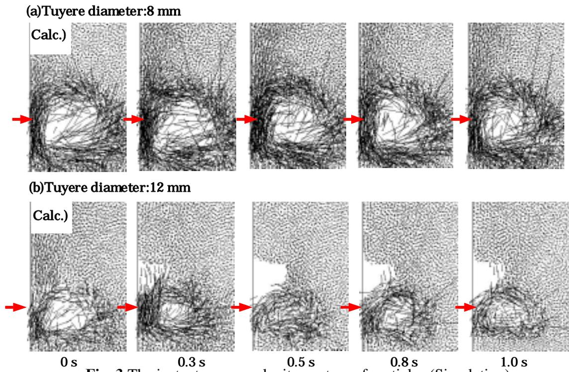
**Fig. 3** The instantaneous velocity vectors of particles (Simulation)
