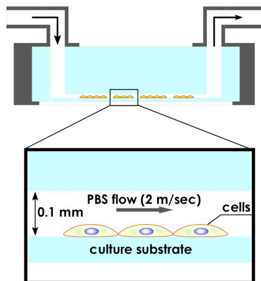
Fig.2. Set up for flushing the surface of culture substrate in a certain flushing condition.
