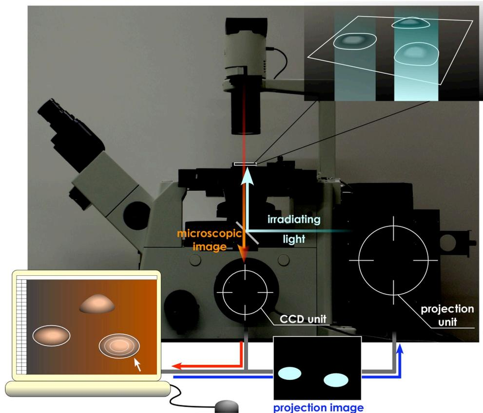
Fig.1. A schematic illustration of the cell manipulation system based on photo- induce cell capturing.
