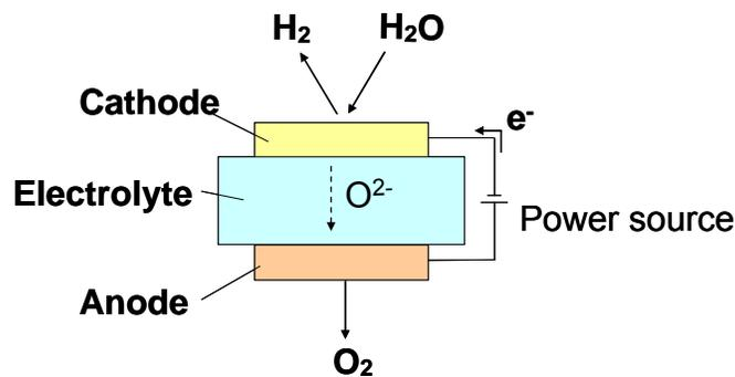
Figure 1 Principle of high temperature electrolysis
