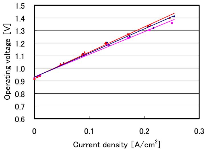
Figure 9 Current-voltage characteristic of fifteen 75 cm<sup>2</sup> cells assembly unit
