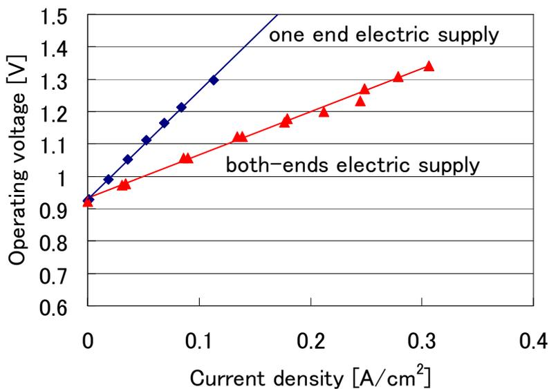
Figure 8 Current-voltage characteristic of  $75 \text{ cm}^2$  cell
