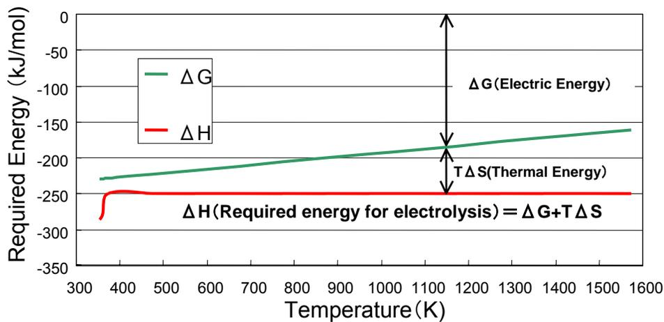
Figure 2 Required Energy for Electrolysis
