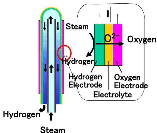
Figure 3 Structure of Tubular Electrolysis Cell
