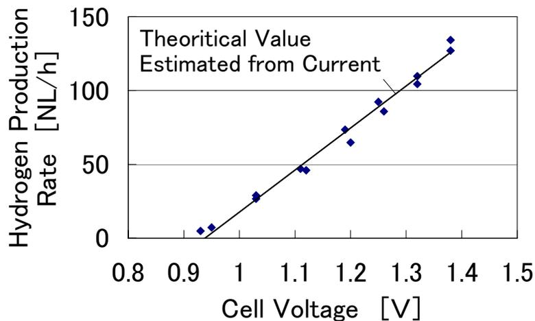
Figure 10 Hydrogen production test result of fifteen 75 cm<sup>2</sup> cells assembly unit
