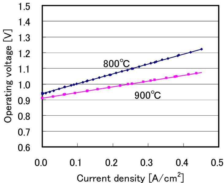
Figure 7 Current-voltage characteristic of 15 cm<sup>2</sup> cell
