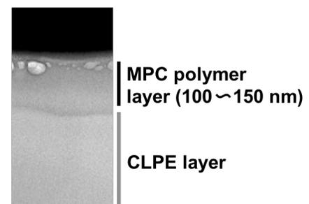
Fig. 3. Cross-section of interface between CLPE layer and MPC polymer layer grafted on the surface
