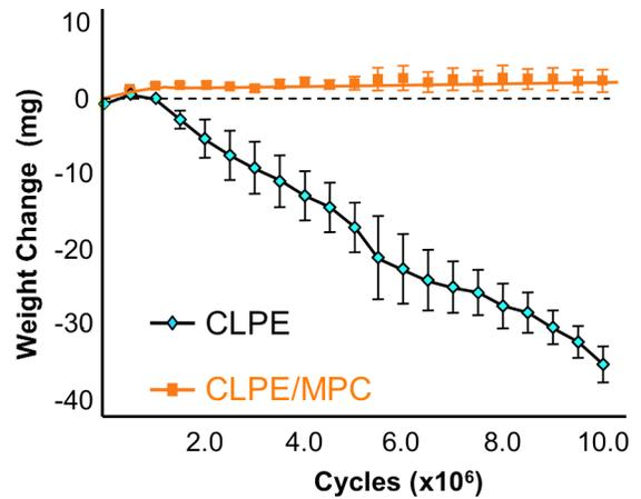
Fig. 4. Wear of CLPE/MPC polymer liners and non-treated CLPE liner during simulation experiments
