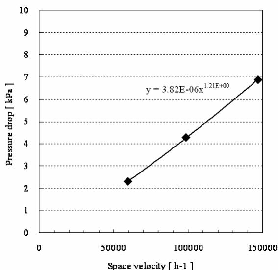
Figure 8 Pressure drop as a function of space velocity
