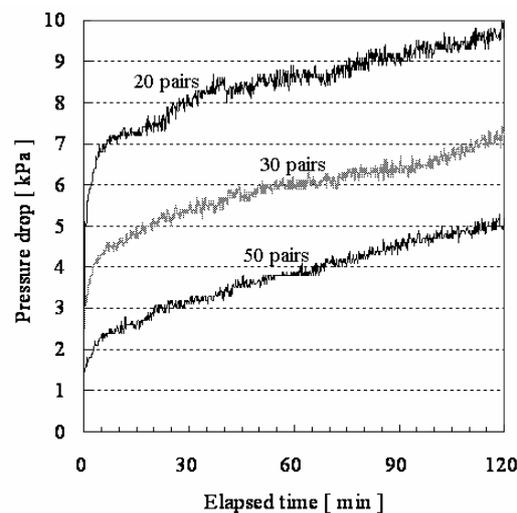
Figure 7 Pressure drop of the uneven DBD reactor.
