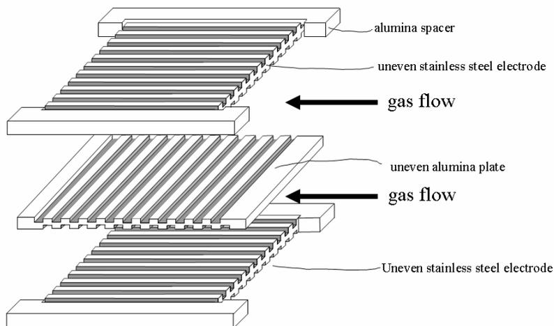
Figure 1 Basic arrangement of uneven alumina plate and stainless steel plate
