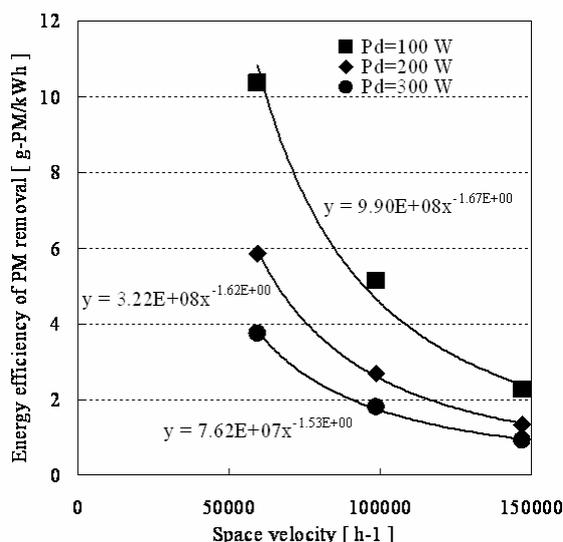
Figure 5 Relationship between energy efficiency of PM removal and space velocity
