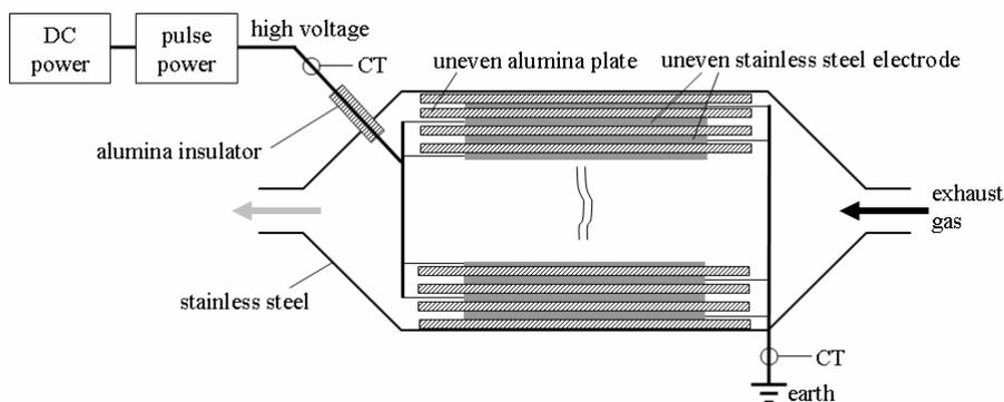
Figure 2 Structure of uneven DBD reactor
