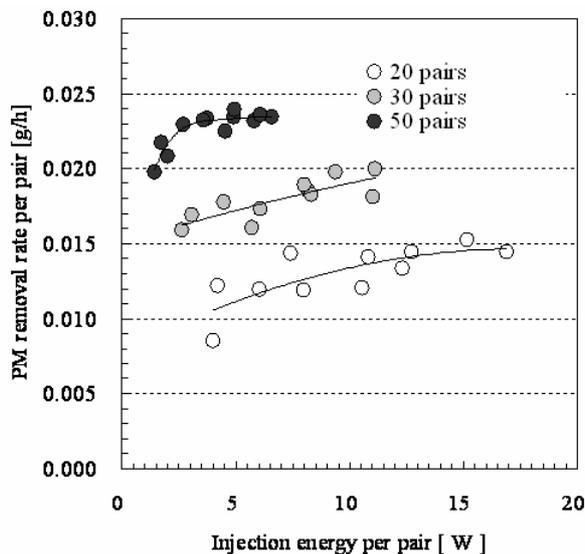
Figure 6 PM removal rate per pair as a function of energy injection to each pair
