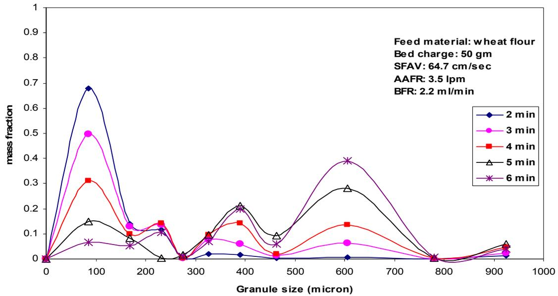
**Fig. 1. Evolution of differential size distribution versus time**
