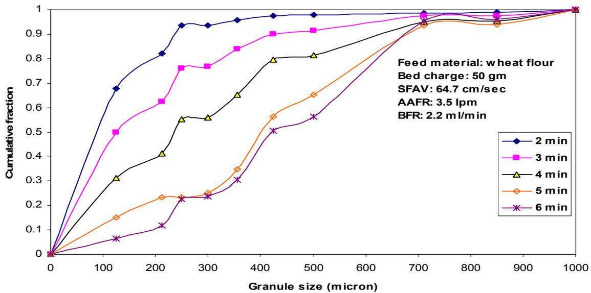
**Fig. 2. Evolution of cumulative particle size distribution versus time**
