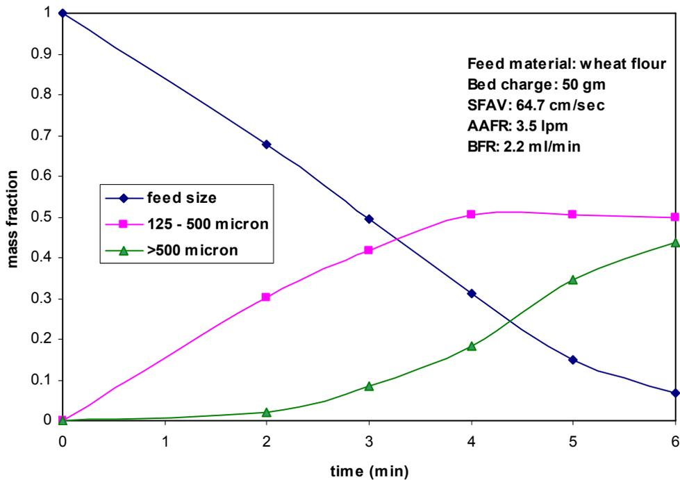
Fig. 3. Evolution of three characteristic classes versus time
