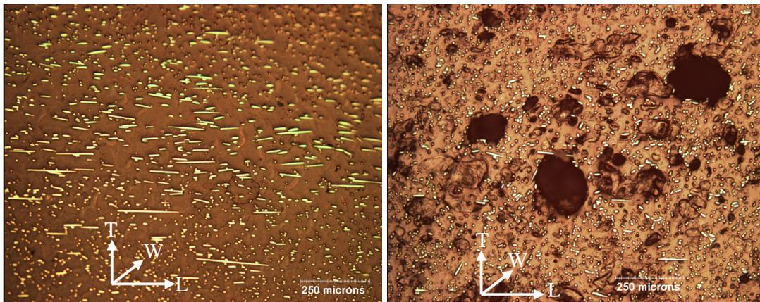
**Fig. 4.** Micrographs from reflected light microscopy showing the fiber orientation distribution of the injection molded composites: Left: non-foamed sample (A) and Right: foamed sample (C)
