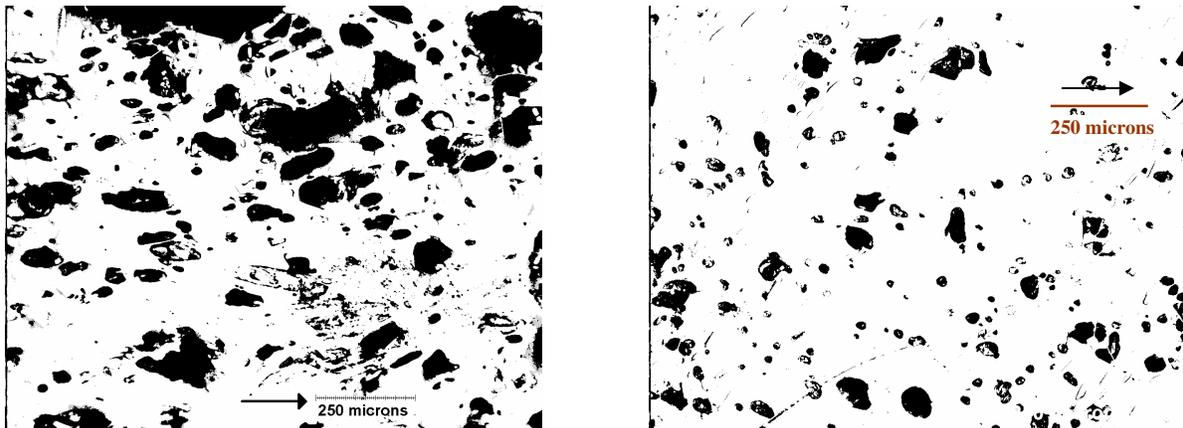
**Fig. 3.** Micrographs of the foam injection molded samples obtained from polished T2B samples by reflected light microscopy: left: run (5) and right: run (6)
