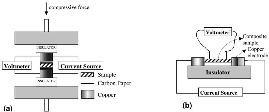
**Fig. 2** Schematic diagram of the set-up for electrical conductivity measurement (a) 2-probe method and (b) 4-probe method
