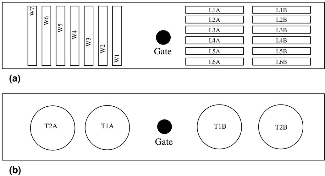
**Fig. 1** Cutting pattern to prepare samples for electrical conductivity measurements: (a) samples for longitudinal and transverse measurements and (b) samples for through-plane measurements
