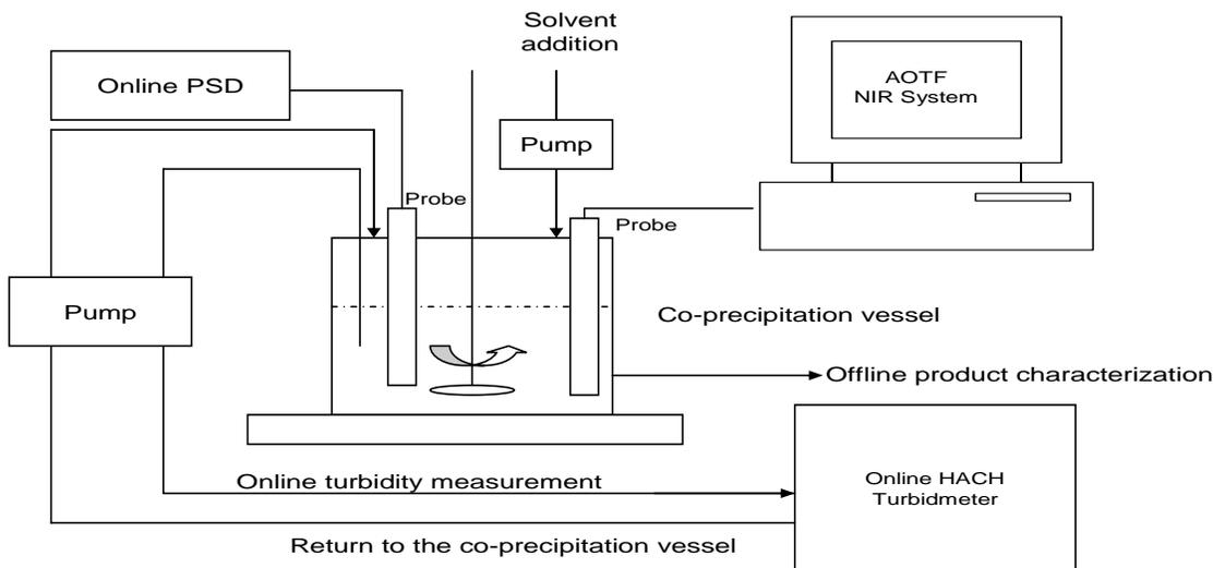
Figure 1. Schematic diagram of experimental setup and process flow system with an on-line PAT monitoring system for pharmaceutical API/polymer co-precipitation process
