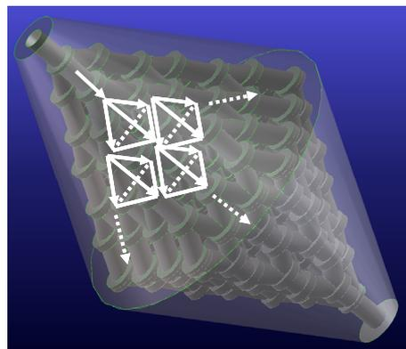
**Figure 1.** A model bioreactor for perfusion culture based on 4-mm-length-edge regular tetrahedrons.
