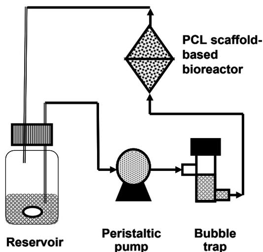
**Figure 2. Scheme of the perfusion circuit system**
