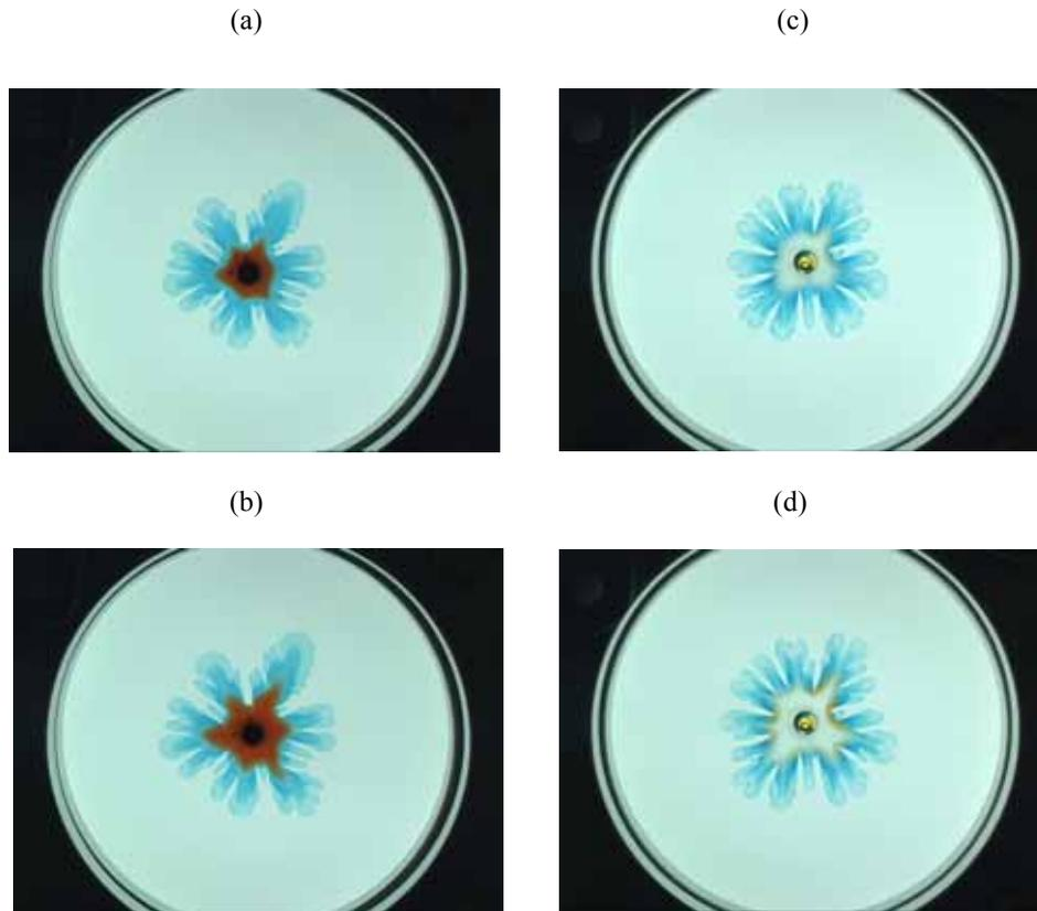
Figure 2. Viscous fingering pattern without and with the reaction when  $t_{sw}=90$  s. (a) without reaction at  $t=120$  s; (b) without reaction at  $t=150$  s; (c) with reaction at  $t=120$  s; (d) with reaction at  $t=150$  s.
