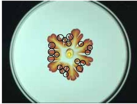
Figure 5. Reaction region in reactive miscible viscous fingering at  $t=150$  s at  $\phi_v=1$  ( $c_{l0}=0.04$  mol/l and  $c_{m0}=0.08$  mol/l) under the condition of  $b=0.3$  mm and  $q=1.8$  mm<sup>3</sup>/s. Blood red color region except the region specified by black circles indicates the reaction region, while the black circles represent the region in which the reaction does not take place although the product exists.
