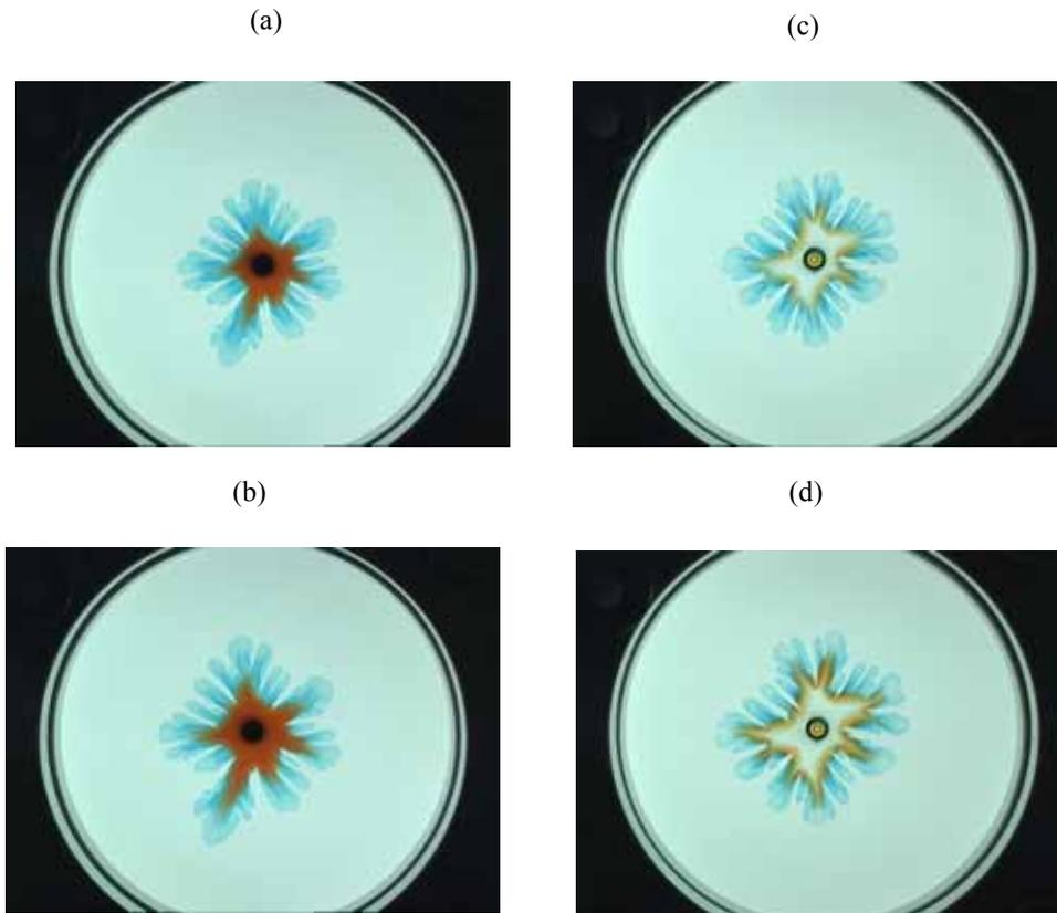
Figure 3. Viscous fingering pattern without and with the reaction when  $t_{sw}=60$  s. (a) without reaction at  $t=120$  s; (b) without reaction at  $t=150$  s; (c) with reaction at  $t=120$  s; (d) with reaction at  $t=150$  s.
