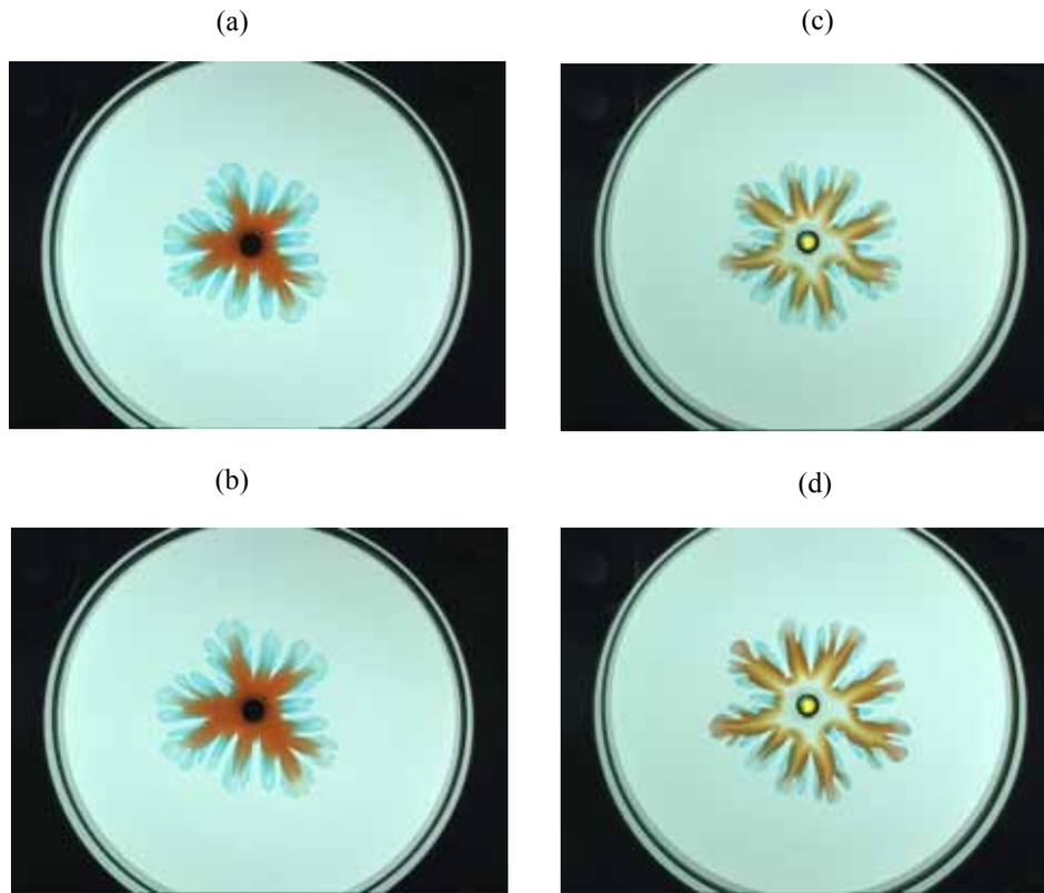
Figure 4. Viscous fingering pattern without and with the reaction when  $t_{sw} = 30$  s. (a) without reaction at  $t = 120$  s; (b) without reaction at  $t = 150$  s; (c) with reaction at  $t = 120$  s; (d) with reaction at  $t = 150$  s.
