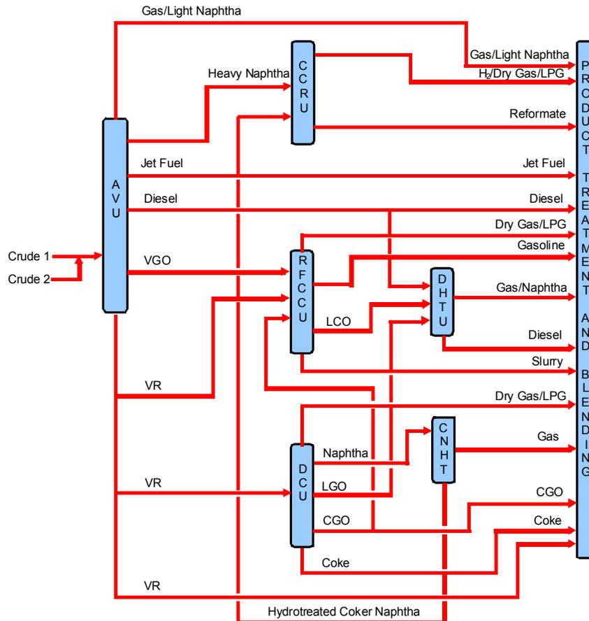
**Figure 2:** Refinery processes connectivity for case study
