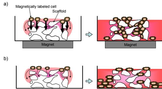
Figure 2. Schematic diagram of Mag-seeding. a) Mag-seeding. b) Static seeding. For Mag-seeding, a magnet is placed at the reverse side of the culture dish and the magnetically labeled cells are attracted by the magnetic force (solid arrow). For static-seeding, the cells are moved by the medium flow (dotted arrow).
