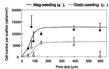
Figure 4. Relationship between pore size and number of cells seeded in each scaffold. Open circles, static-seeding; closed circles, Mag-seeding. Data points represent mean  $\pm$  SD of triplicate experiments.
