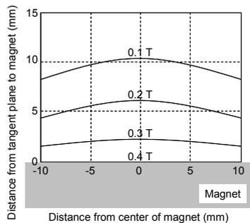
Figure 5. Magnetic flux of 0.4 T magnet. Constant magnetic flux density lines from the surface of the 0.4 T magnet are shown. Magnetic flux was measured using a handheld gauss meter.
