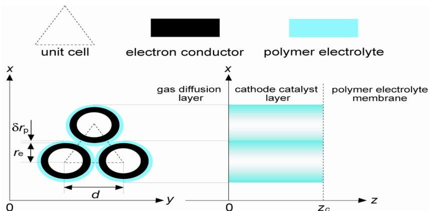
**Figure 1** Schematic diagram of an ordered catalyst layer in a PEMFC cathode.
