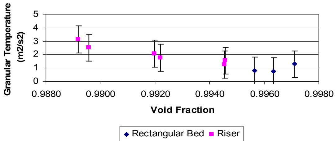
Figure 7. Granular Temperature For Riser and Rectangular Bed Experiments
