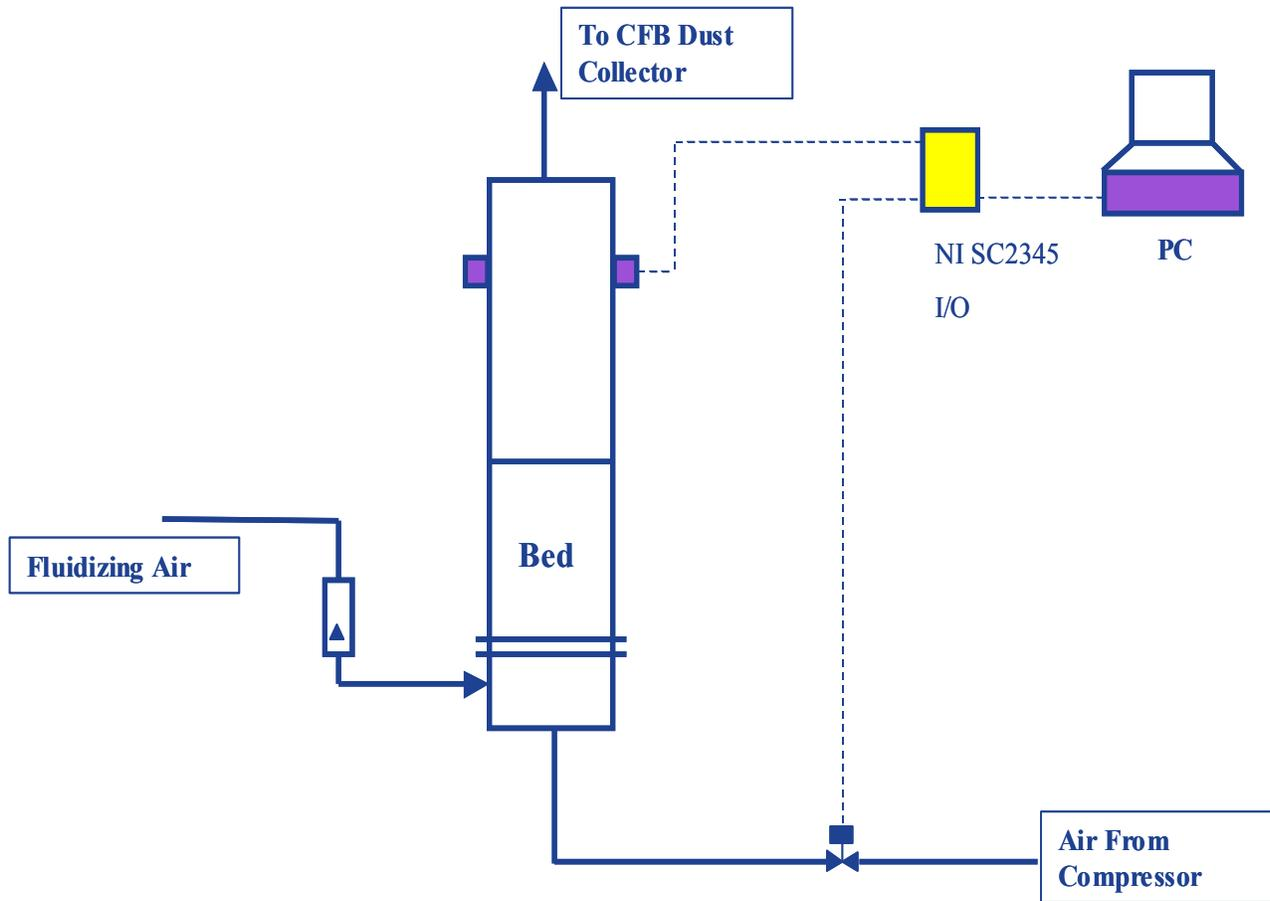
Figure 1. Schematic Diagram for Riser Experiments
