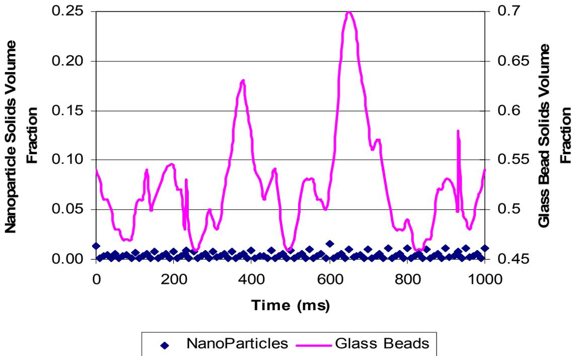
Figure 4. Solids Volume Fraction Variation For Nanoparticles and Glass Beads
