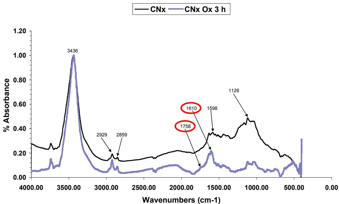
**Figure 3.** Infrared spectrum for CNx before and after its functionalization with  $\text{HNO}_3$
