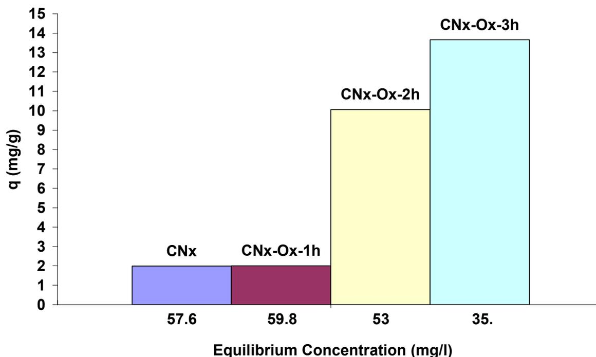
**Figure 4.** Cadmium adsorption capacity of CNx. Initial concentration of 60 mg/L, pH 6, and 25° C.
