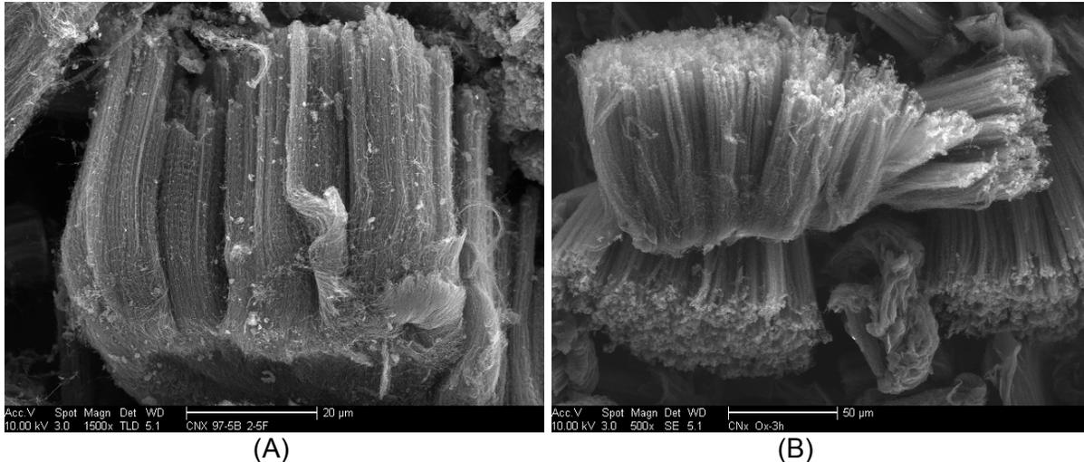
**Figure 1.** (A) Micrograph of CNx synthesized; (B) Micrograph of CNx modified for 3 h
