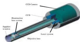
Particle Vision and Measurement (PVM) is *in situ* video microscopy that captures and records pictures of a system in real time avoiding the need for countless stage microscope samples and the ability to save all captured micrographs electronically.
