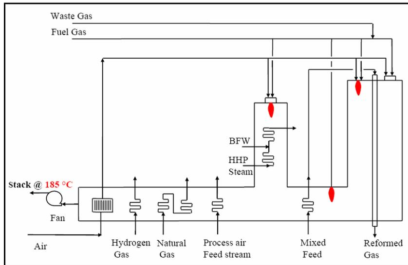
**Fig. 10:** The coil arrangement of the existing plant
