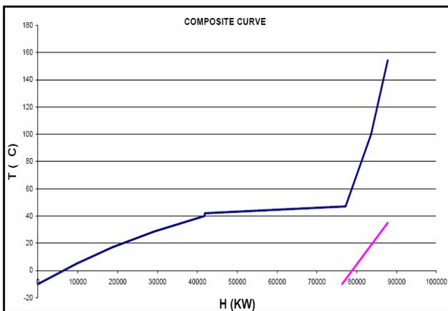
Fig 16: Composite Curve of cold section cold section
