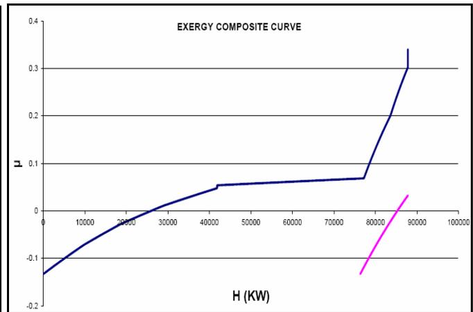
Fig 17: Exergy Composite Curve of cold section
