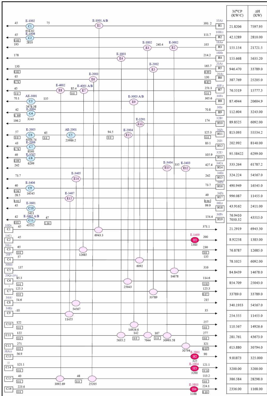
Fig.4: Grid diagram of the existing HEN proposed for the hot section
