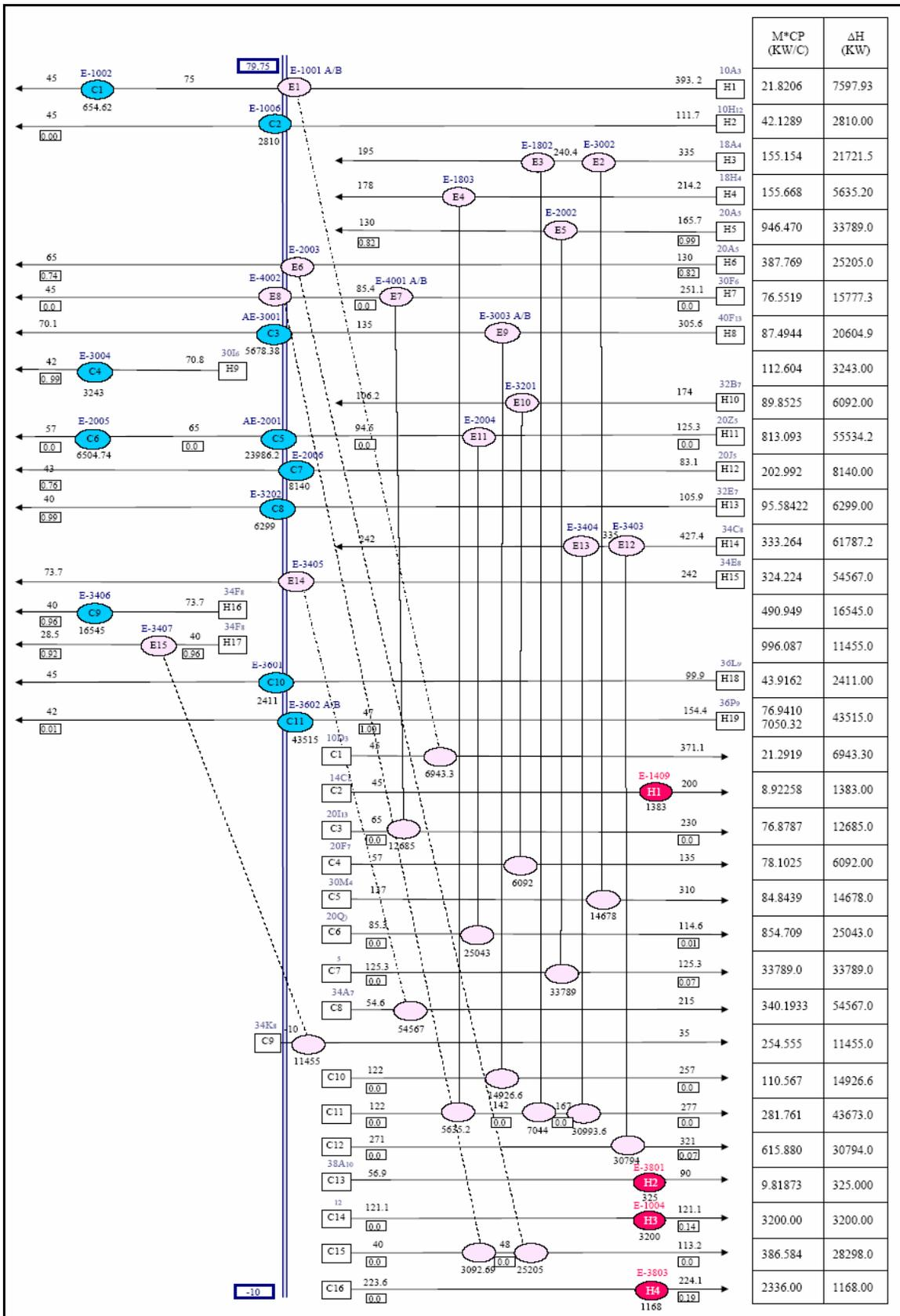
Fig. 7: Grid diagram of existing HEN corresponds to Cold P.H.
