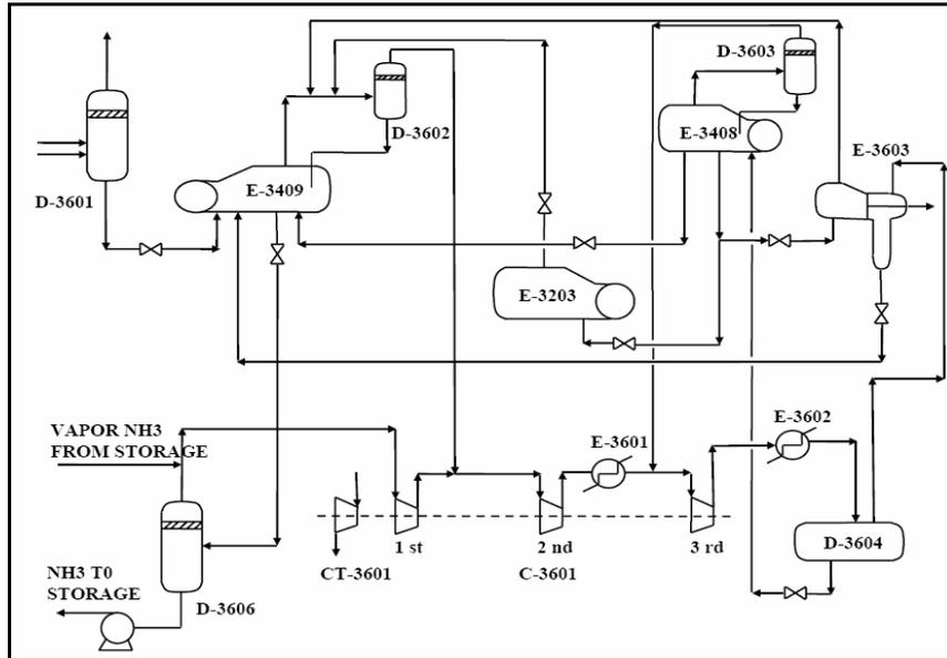
**Fig 14:** Schematic of ammonia refrigeration cycle
