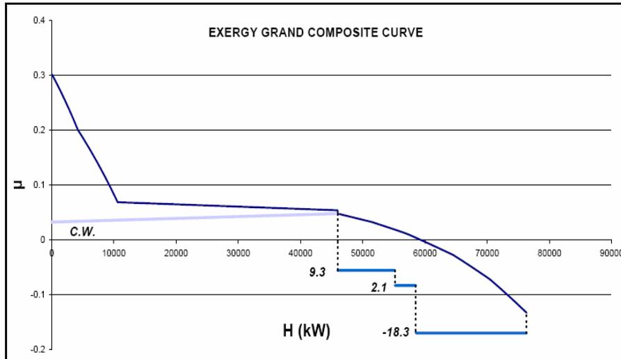
**Fig 18:** The refrigeration level placements on the Exergy Grand Composite Curve for existing refrigeration cycle
