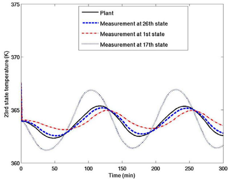
Fig. 9. Reconstruction of 23rd state in the distillation column, for optimal (26<sup>th</sup> tray) and non-optimal ( 1<sup>st</sup> and 17<sup>th</sup>), for sinusoidal process disturbance of 10% in the feed composition
