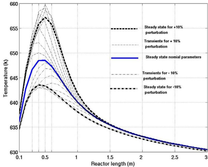
Fig.3. Steady state and transient profile for nominal feed composition and  $\pm 10\%$  disturbance in the feed composition
