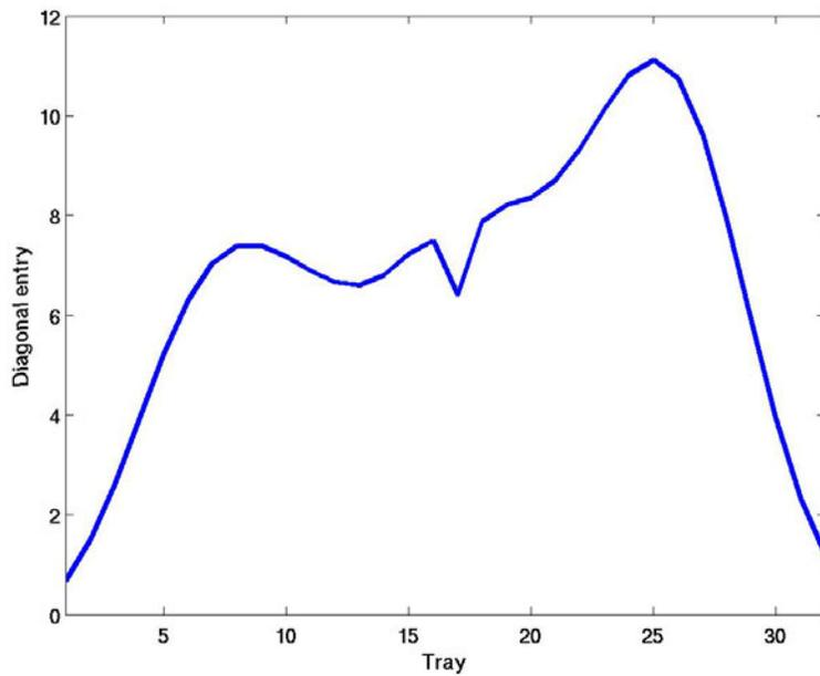
Fig. 5. Diagonal entry of states (variance of states) in the empirical controllability gramian for 10% disturbance in feed composition for the distillation column
