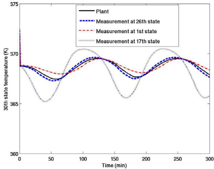
Fig. 10. Reconstruction of 30<sup>th</sup> state in the distillation column, for optimal (26<sup>th</sup> tray) and non-optimal (1<sup>st</sup> and 17<sup>th</sup>), for sinusoidal process disturbance of 10% in the feed composition
