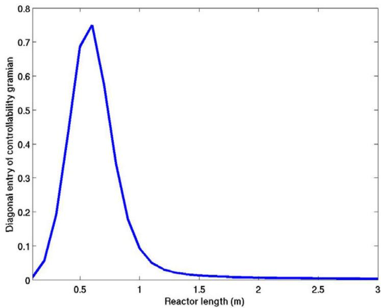
Fig. 2. Diagonal entry of states, i.e. variances of the states, in the empirical controllability gramian for 10% disturbance in feed composition for the fixed bed reactor
