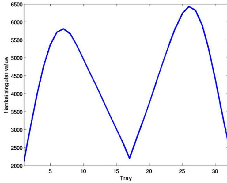
Fig. 6 Measure for placing one sensor in the distillation column with 10% disturbance in feed composition
