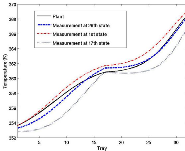
Fig. 11. Reconstruction of distillation column profile, for optimal (26<sup>th</sup> tray) and non-optimal (1<sup>st</sup> and 17<sup>th</sup>), for 10% step disturbance in the feed composition
