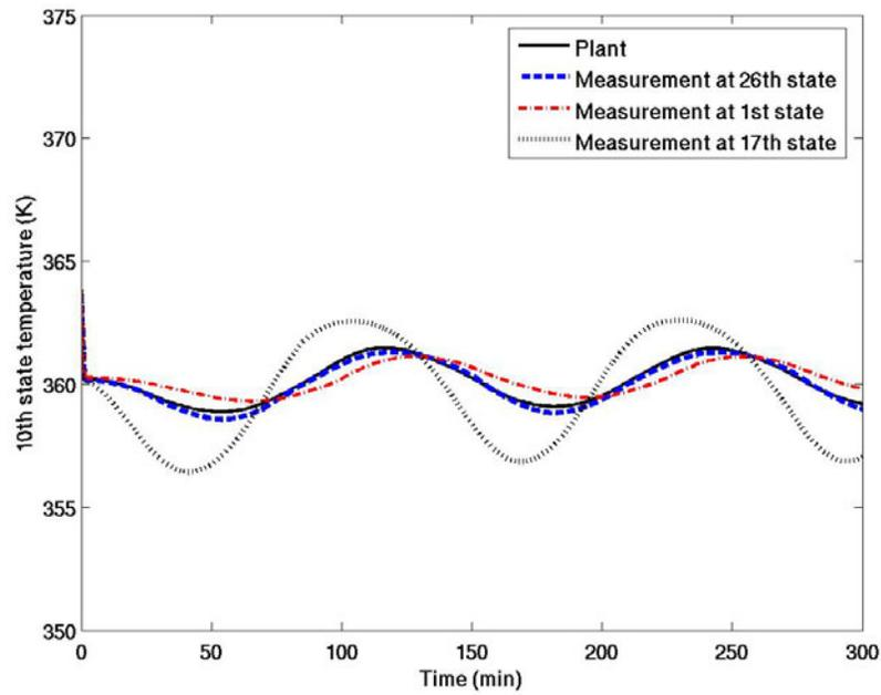
Fig. 8. Reconstruction of 10<sup>th</sup> state in the distillation column, for optimal (26<sup>th</sup> tray) and non-optimal ( 1<sup>st</sup> and 17<sup>th</sup>), for sinusoidal process disturbance of 10% in the feed composition
