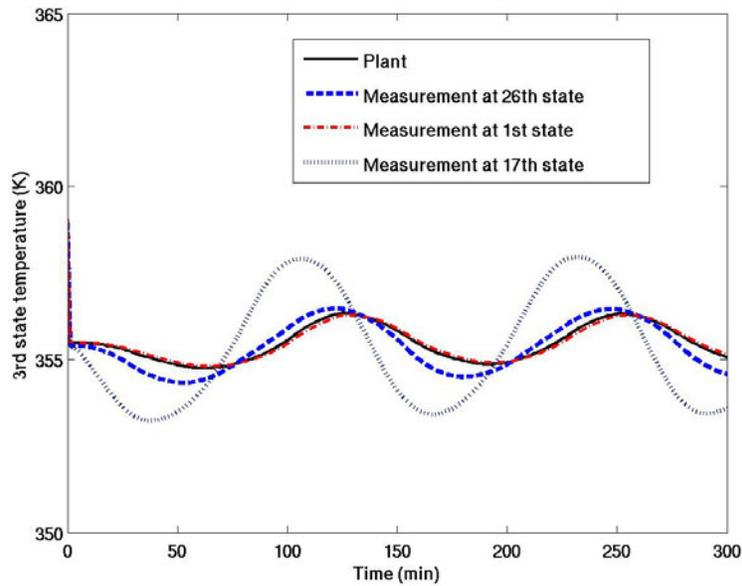
Fig. 7. Reconstruction of 3<sup>rd</sup> state in the distillation column, for optimal (26<sup>th</sup> tray) and non-optimal ( 1<sup>st</sup> and 17<sup>th</sup>), for sinusoidal process disturbance of 10% in the feed composition
