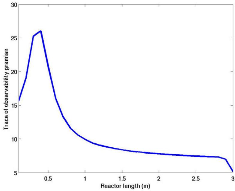
Fig. 4. Measure for placing one sensor in the reactor for nominal operating parameters
