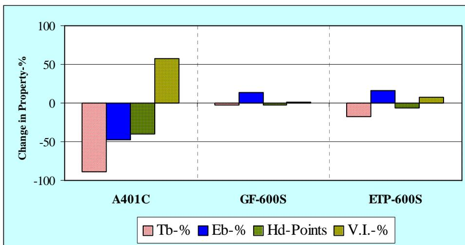
\*ASTM D412: Tb = Tensile Strength, Eb = Elongation    ASTM D2240: Hd = Hardness, Shore A
