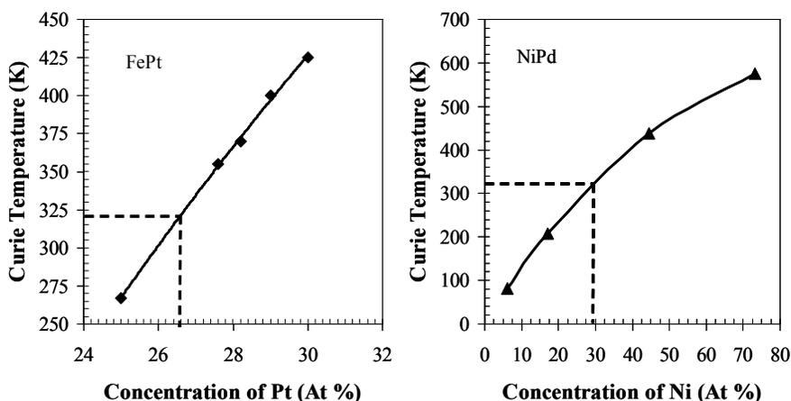
Figure 1.  $T_c$  plots of bulk FePt<sup>28</sup> and NiPd<sup>29</sup> alloys in the disordered fcc state as a function of their composition.
