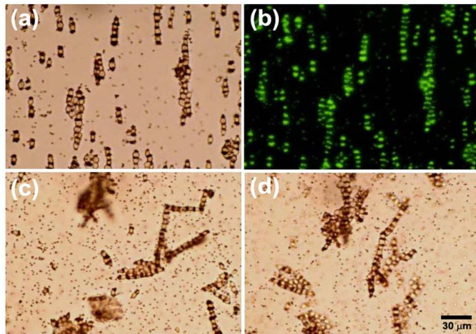
**Figure 3.** Cell chains obtained using fluorescent lectin conjugated flouraldehyde latex. (a) & (b) complementary images of striped “tiger-like” chains formed from 0.2 wt% cells and 0.1 wt% particles in AC electric fields of 30 V, 200 Hz. The final protein concentration obtained in the solution was 0.05 mg lectin/mg latex. (c) & (d) AC field ‘off’. Chains develop hinges after perturbation. The images indicate rigidity of the chains.
