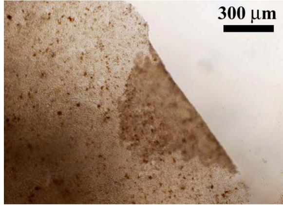
Fig. 4. A folded magnetic membrane of yeast cells. The membrane is a matrix of cells and lectin-coated magnetic nanoparticles.
