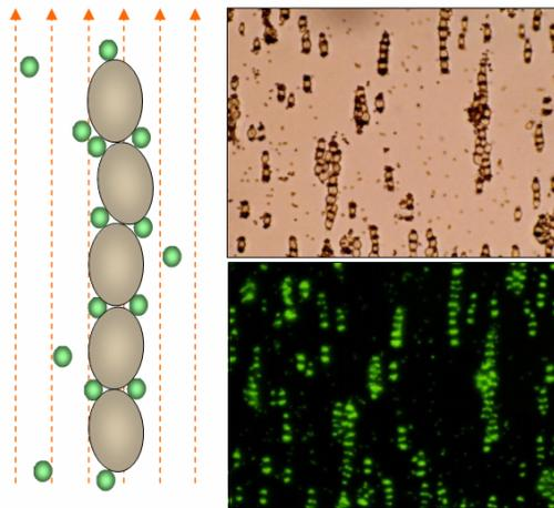
**Figure 1.** Assemblies of yeast cells and 1  $\mu\text{m}$  fluorescent microparticles made by AC electric field. The specific organization of the particles in the junction between the cells (compare the regular and fluorescence images) occurs because of the induced dipolar interactions.
