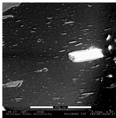
Figure 13: ESEM Image showing the orientation and agglomeration of xGnP-15 in 1 vol% xGnP-15/PP composite made by melt mixing and injection molding (scale bar 500  $\mu\text{m}$ )
