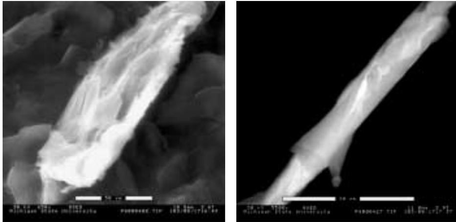
Figure 12: ESEM Image of a) graphite agglomerate in a 1 vol% xGnP-15-PP (scale bar 50  $\mu\text{m}$ ) and b) “roll-up” of xGnP-15 in 1vol% xGnP-15-PP (scale bar 10  $\mu\text{m}$ )
