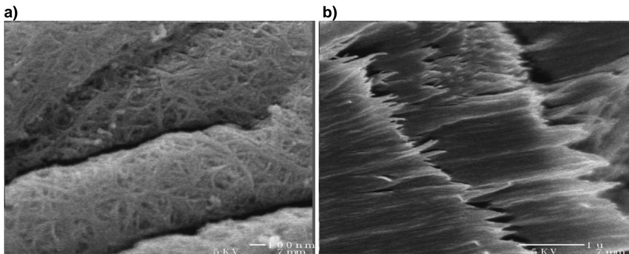
**Fig. 4** Scanning electron microscopy (SEM) of material after 24 h reflux with 6 N HCl.
