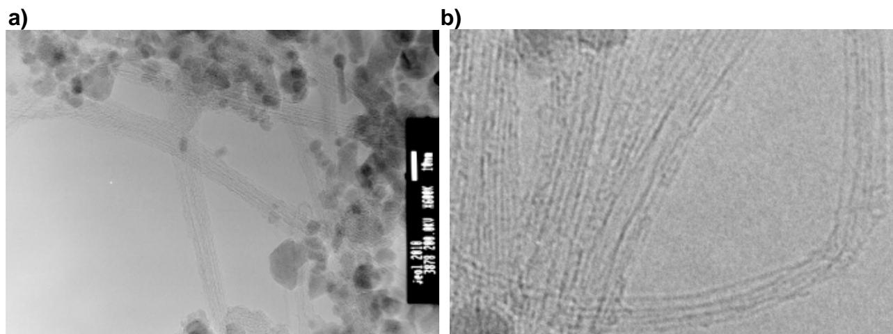
**Fig. 3** Transmission electron microscopy (TEM) of as-produced material.
