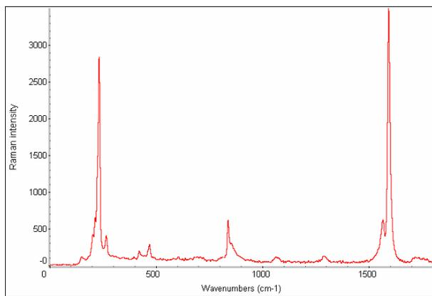
**Fig. 1** Raman spectrum of as-produced combustion-generated material. 785 nm.
