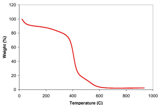
**Fig. 5** Thermogravimetric analysis (TGA) of combustion-generated SWCNT material after 24 h reflux in 3 N HNO<sub>3</sub>.
