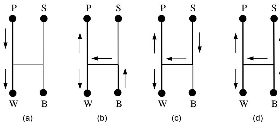
**Figure 4:** The sequential steps of the immunoassay. Solution delivery occurs in the dark colored channels whereas in the light colored channels, the solution is almost stagnant. The arrows indicate the flow direction. (a) dispensing and incubation of the primary antibody; (b) washing of the primary antibody; (c) dispensing and incubation of the secondary antibody; (d) washing of the secondary antibody.
