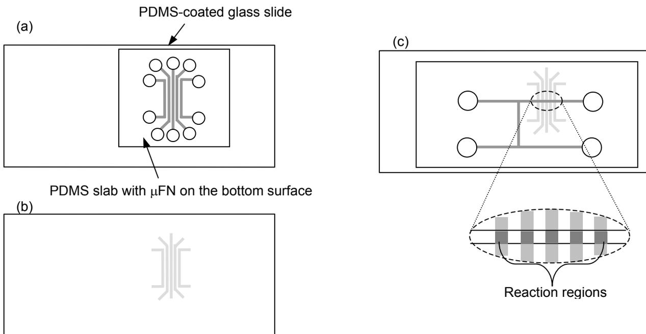
**Figure 3:** The preparation process of the immunoassay (schematics are not proportional to actual size). (a) antigen immobilization using the parallel straight channel  $\mu$ FN; (b) antigen molecules patterned on the surface after a 15-minute immobilization; (c) H-shaped  $\mu$ FN put across the antigen pattern. The intersections of the parallel regions of antigen coating and the H-shaped  $\mu$ FN became reaction regions in later immunoassay experiments.
