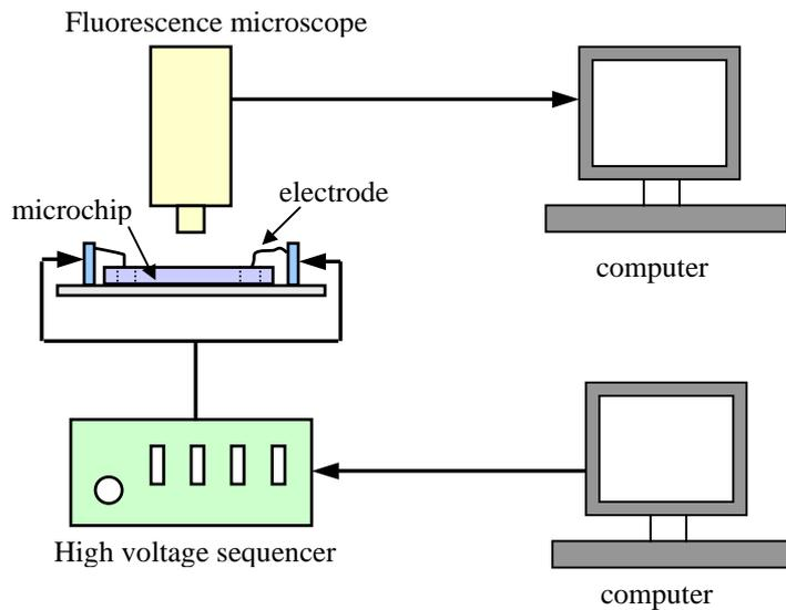
**Figure 2:** A schematic of the experimental setup and imaging system.
