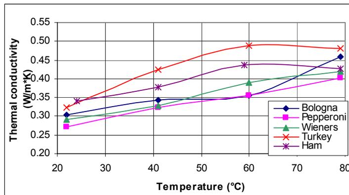
Figure 1: Thermal conductivity of various meat and poultry emulsions at various temperatures.
