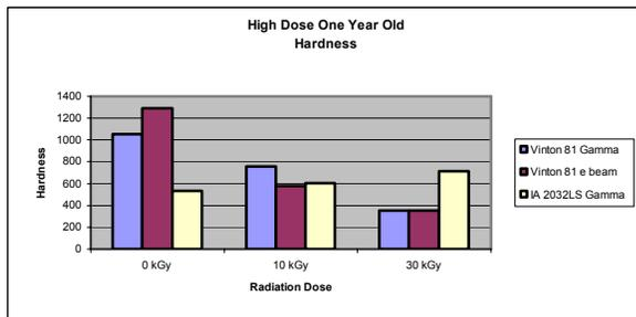
**Figure 13.** Influence of high dose irradiation and storage of soybeans on the hardness of their tofus.
