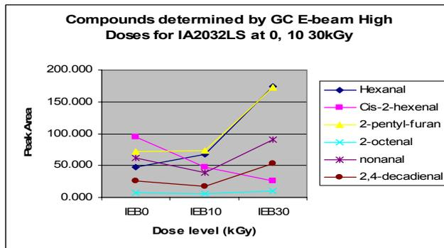
**Figure 7.** Volatile compounds determined by gas chromatography in electron beam irradiated IA2032LS cultivars at 0, 10, 30kGy.
