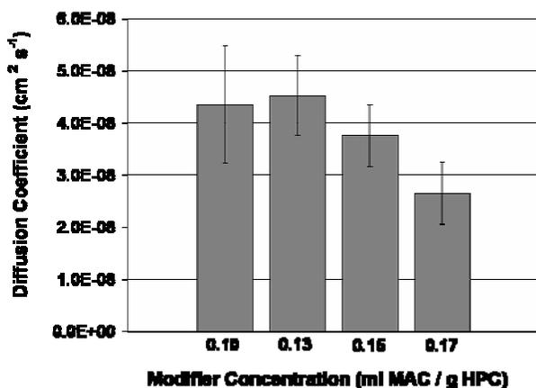
Figure 8: Diffusion coefficients for benzaldehyde through hydrated bulk crosslinked HPC films. The diffusion coefficient decreases as the modifier concentration increases.
