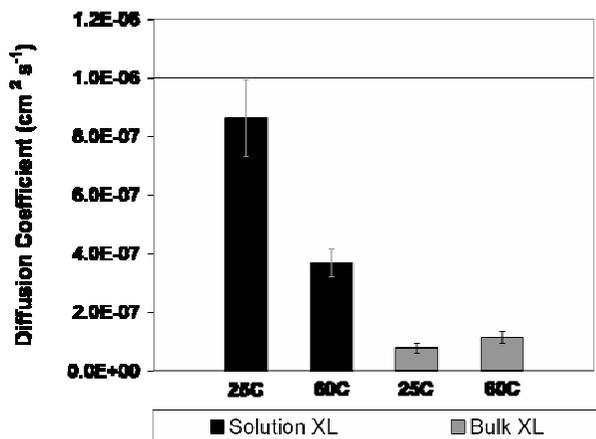
Figure 7: Diffusion coefficients for benzaldehyde through hydrated solution crosslinked and bulk crosslinked HPC films at 25°C and 60°C
