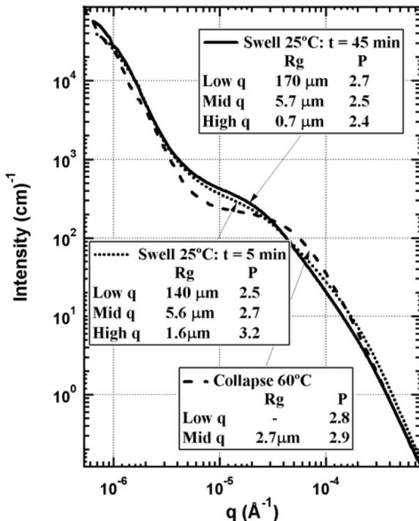
Figure 5: Light scattering data of gel microcapsules indicated three length scales large (low q), overall capsule size; intermediate (mid q), oil containing pores; and small (high q), polymer struts and voids.
