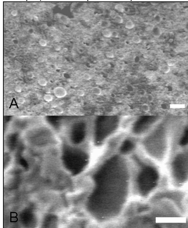
Figure 6: SEM images of a cross sectioned microcapsule. A: Low resolution image at 100x and a scale bar of 50 μm. B: High resolution image at 25,000x and a scale bar of 0.5 μm. Both images reveal porous morphology.
