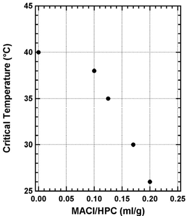
Figure 4: Depression of lower critical solution temperature as the amount of modification increases.
