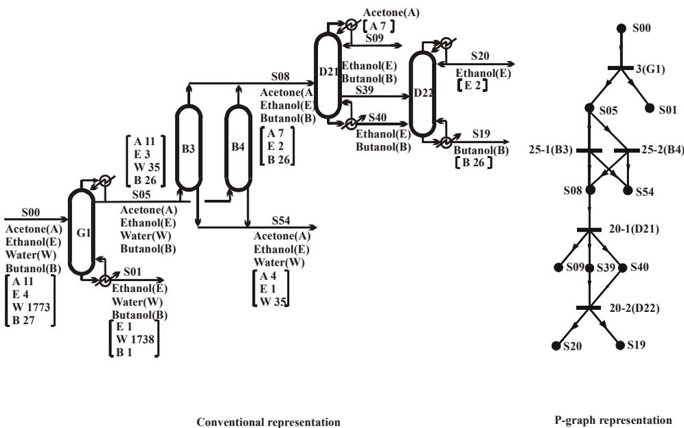
Figure 2. Optimal flowsheet with the consideration of adsorption.
