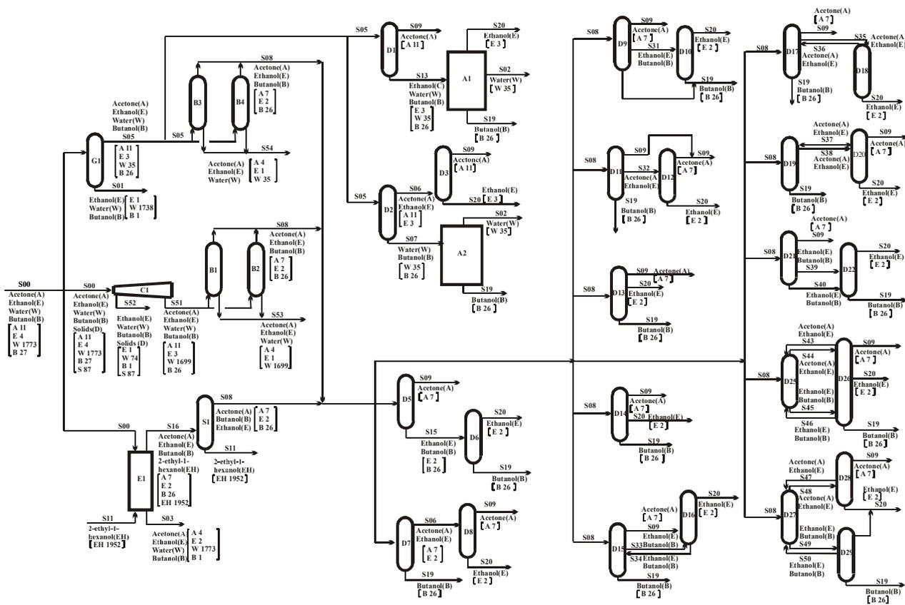
Figure 1. Comprehensive flowsheet corresponding to the maximal structure for the production of butanol, ethanol, and acetone with the inclusion of adsorption: conventional representation.
