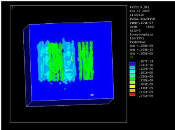
**Figure 1. Finite element model of wave propagation in YZ LiNbO<sub>3</sub>.**
