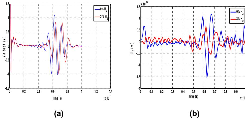
**Figure 2. Voltage and surface normal displacement (U<sub>z</sub>) profile with and without hydrogen adsorbed at the output IDT.**
