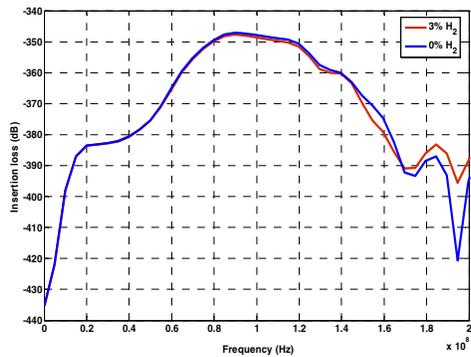
**Figure 4. Frequency response with and without hydrogen adsorbed.**
