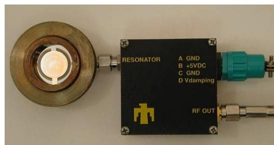
**FIGURE 2.** Sandia national laboratories' oscillator circuit and TSM fixture used in this work
