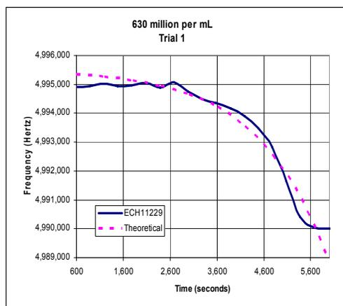
Figures 4 and 5. Frequency response to 630 million unit concentration of *E. coli* growth on TSM device with agar thin film
