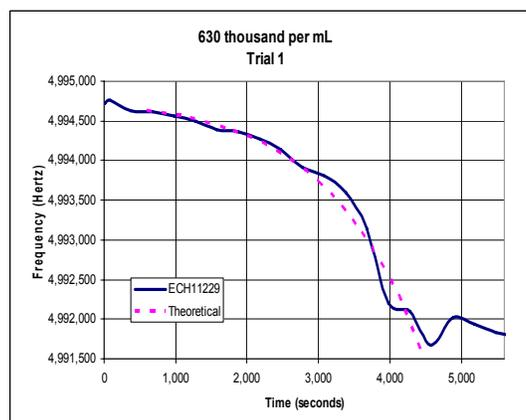
Figure 6. Frequency response to 630,000 unit concentration of *E. coli* growth on TSM device
