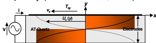
**Figure 3.** Schematic of TSM device with resonating wave
