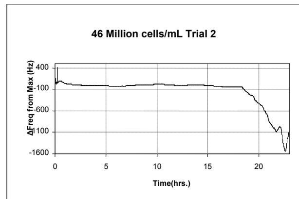
**Figure 8.** Frequency response to 2.5 mL of 46 million cells/mL sample.
