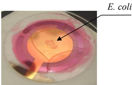
**Figure 9.** 2x magnification of bacterial growth on sensor.
