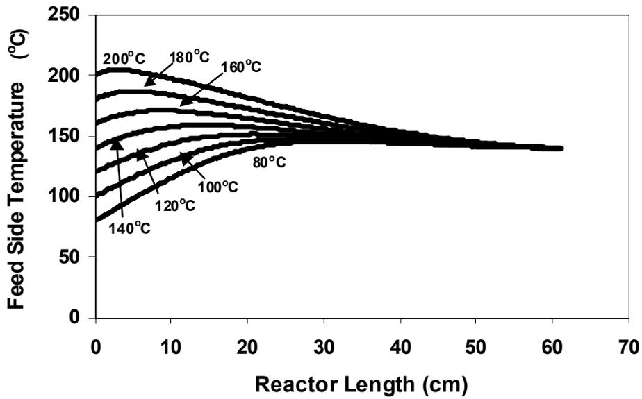
Figure 2. Feed-side temperature profiles along the length of membrane reactor with different inlet feed temperatures.
