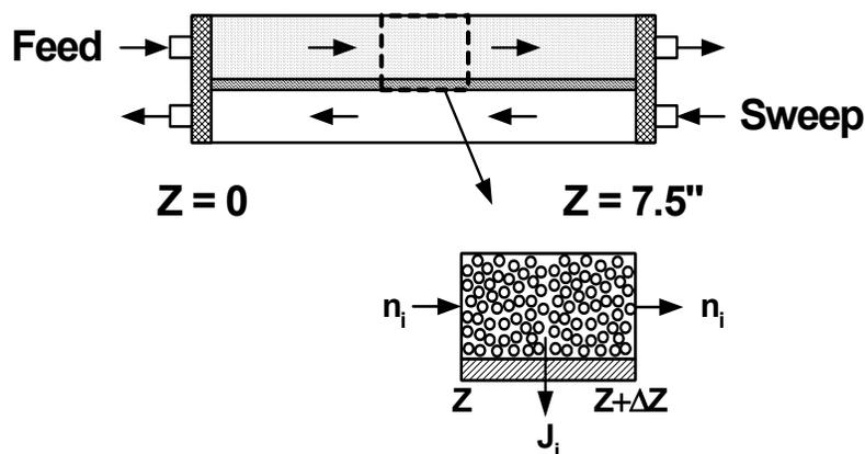
Figure 5. Schematic diagram of flat-sheet WGS membrane reactor
