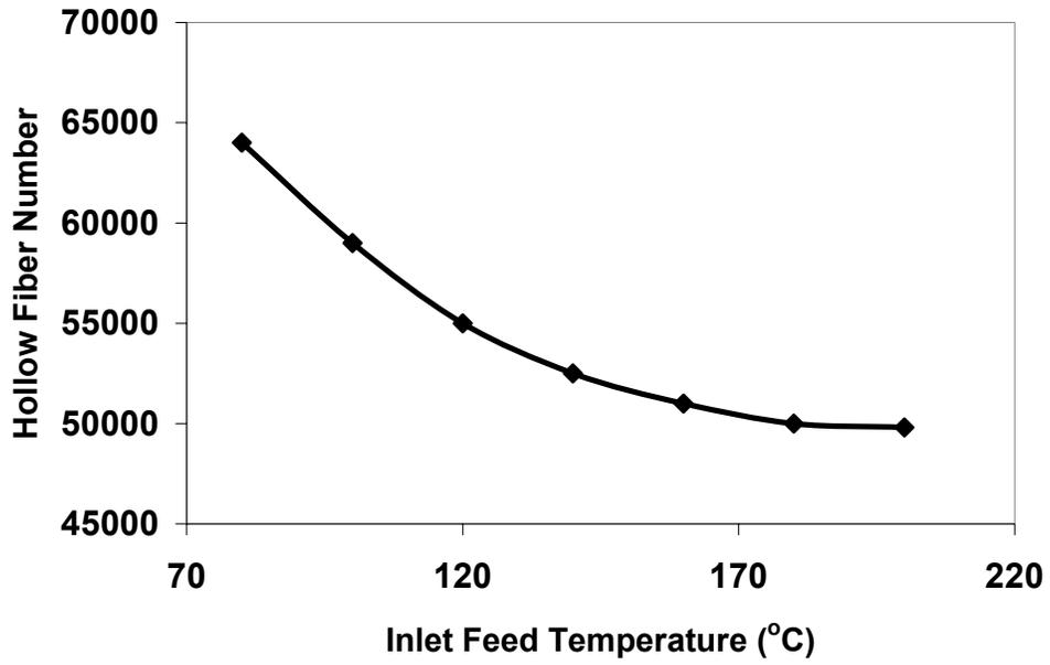
Figure 1. The effect of inlet feed temperature on required membrane area.
