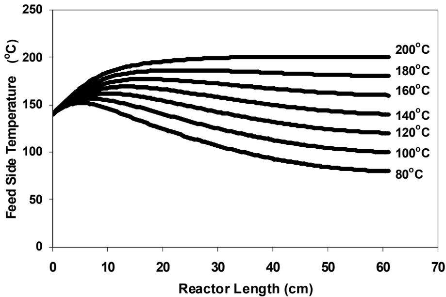
Figure 4. Feed-side temperature profiles along the length of membrane reactor with different inlet sweep temperatures.
