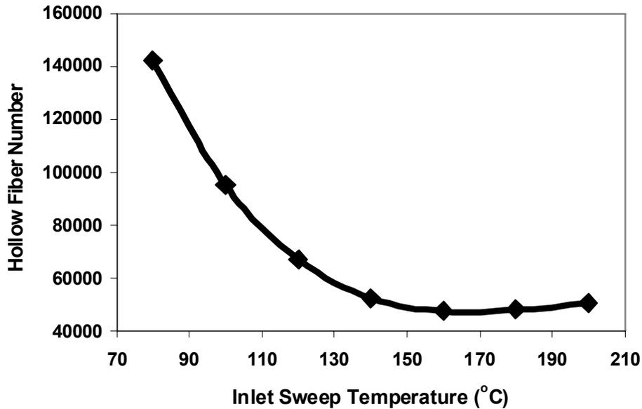
Figure 3. The effect of inlet sweep temperature on required membrane area.
