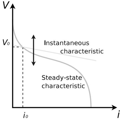
Figure 3: The steady-state polarisation curve and the instantaneous characteristic on a  $V$ - $i$  plane. The instantaneous characteristic can move up or down according to the value of overvoltage  $\eta$ .
