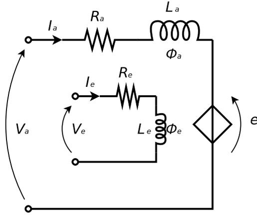
Figure 10: A typical model of a DC motor [20].
