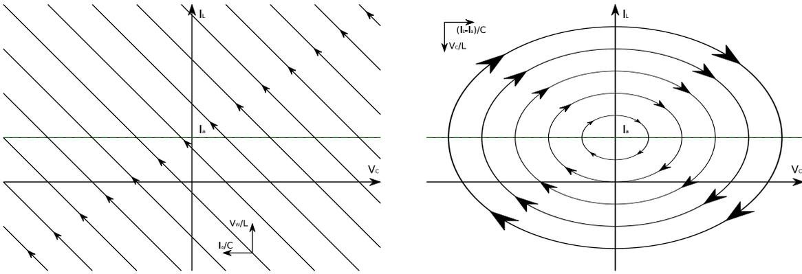
Figure 7: The trajectories of the state variables in a buck-boost converter in the  $V_C-I_L$  plane. On the left-hand side, energy is collected from the input by the inductor. On the right-hand side, no energy is drawn from the source, and the energy stored in the inductor is exchanged with the capacitor. The capacitor delivers power to the output in both configurations. In a real system, the trajectories in the right-hand sides would be spirals, because of losses in the switches.
