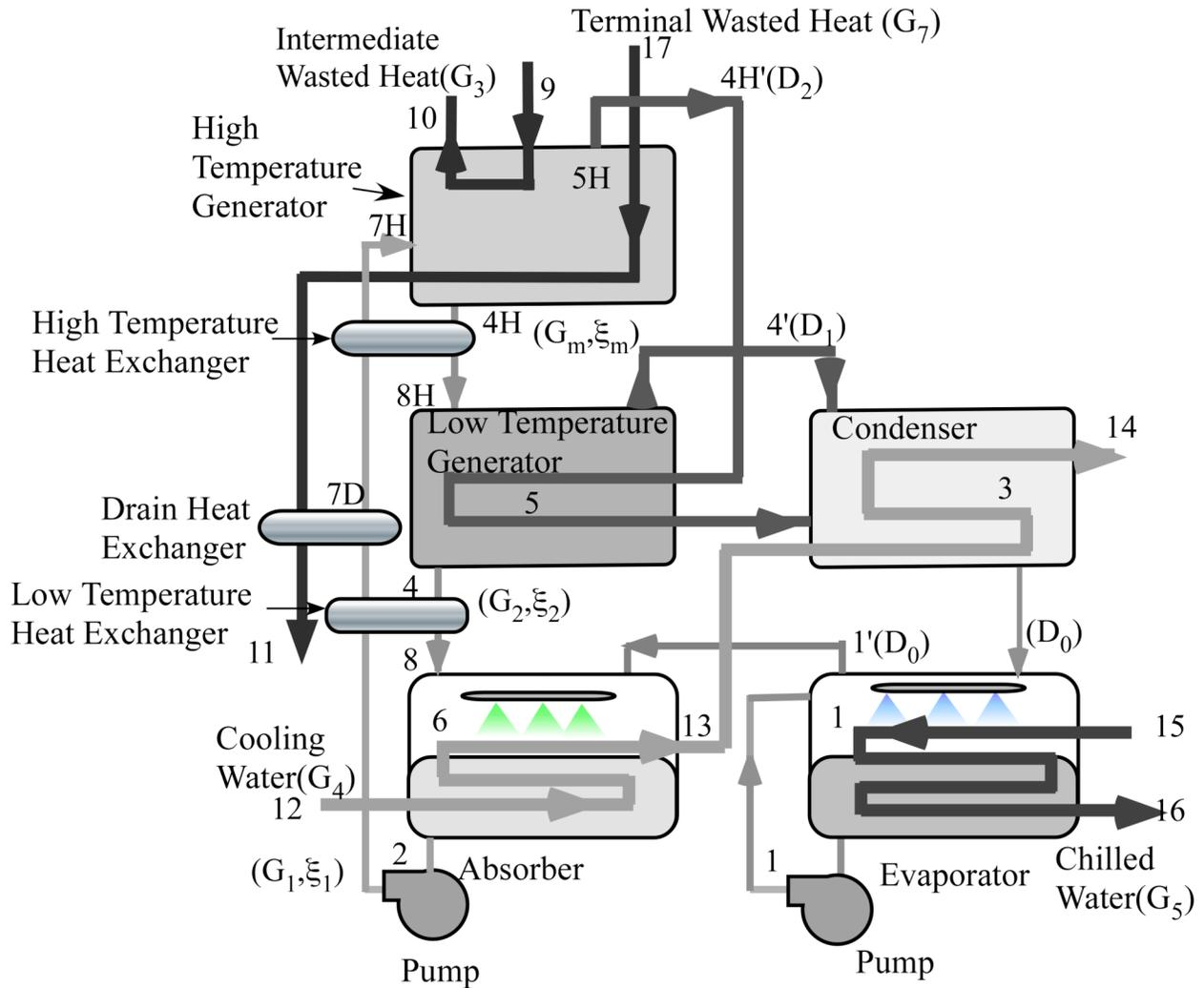
Fig.4 System schematic of series flow on double effect absorption chiller
