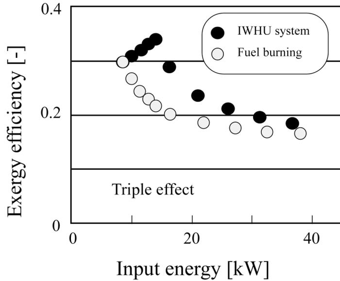
Fig.14 Exergy efficiency of absorption chiller
