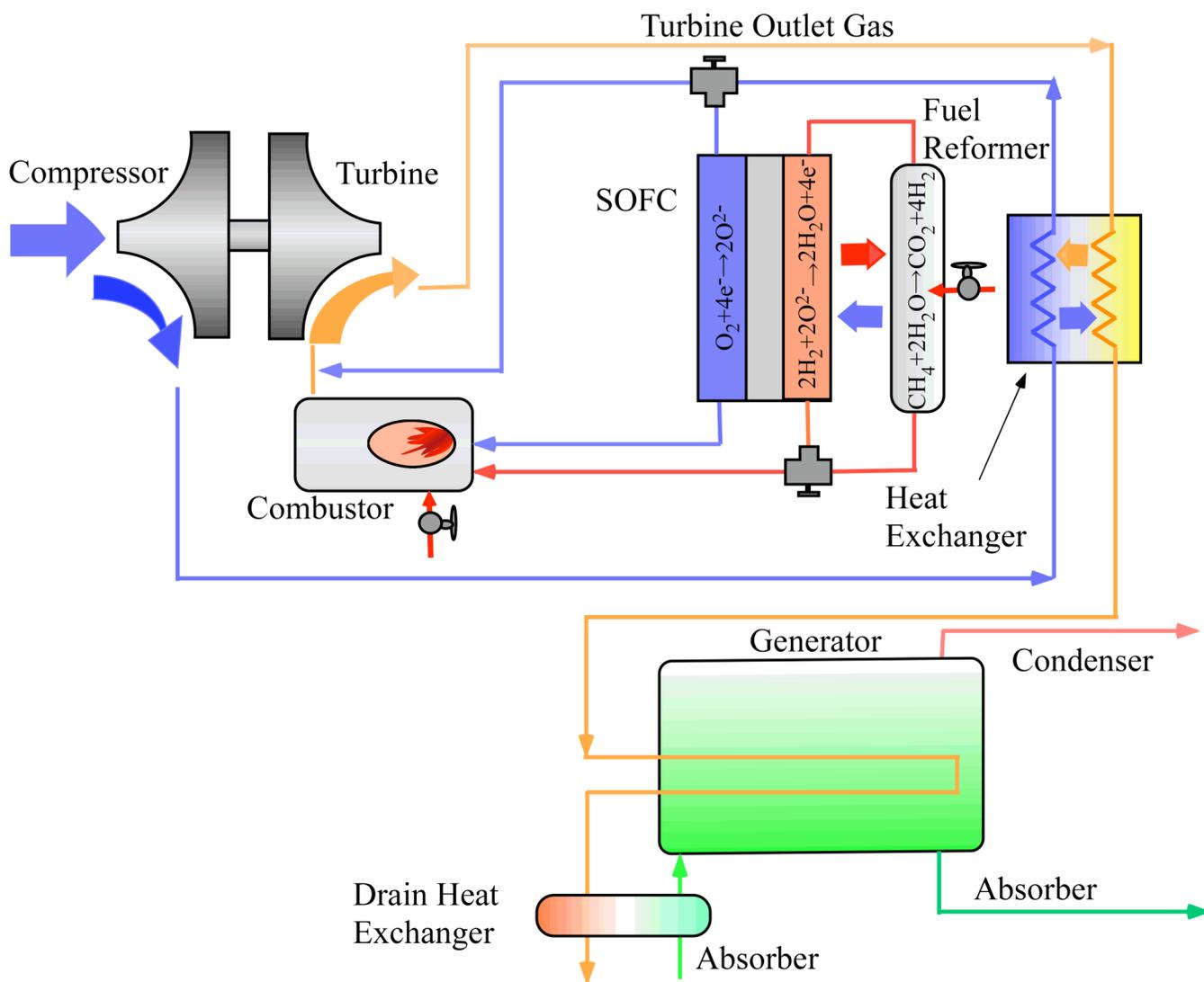
Fig.1 Terminal wasted heat utilization system
