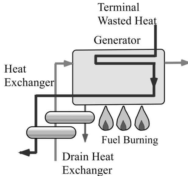
Fig.11 Fuel burning absorption chiller
