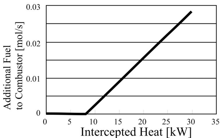
Fig.6 Additional fuel to combustor
