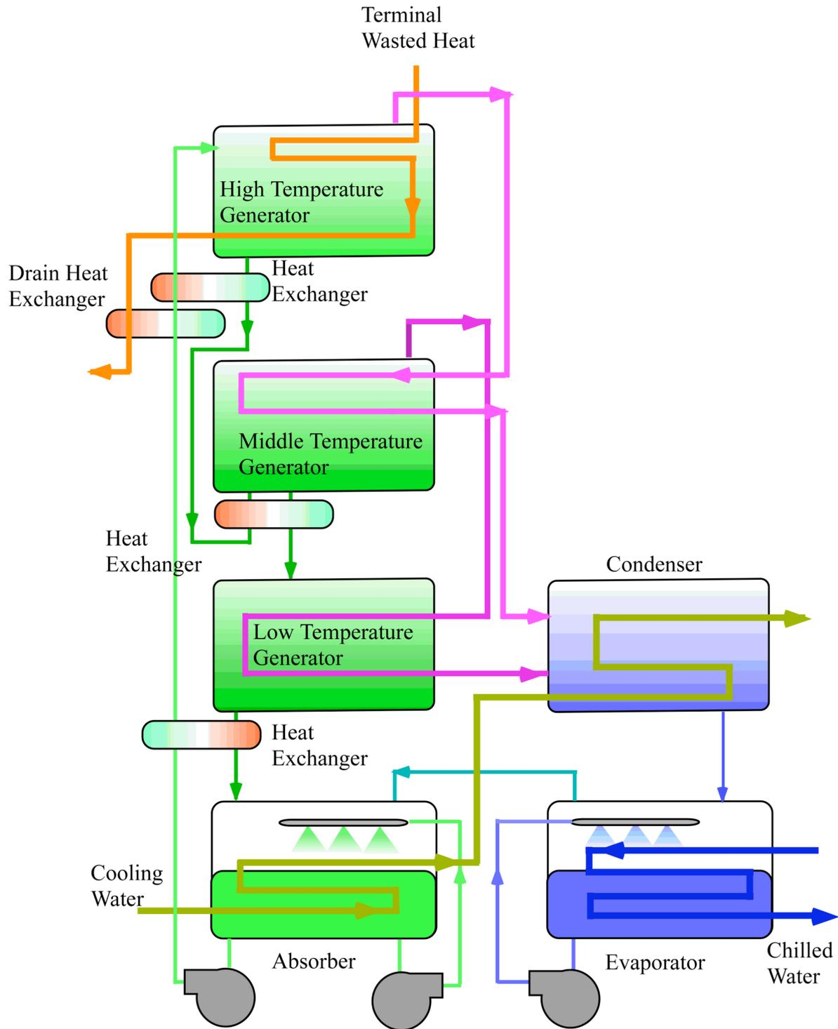
Fig.3 Triple effect absorption chiller
