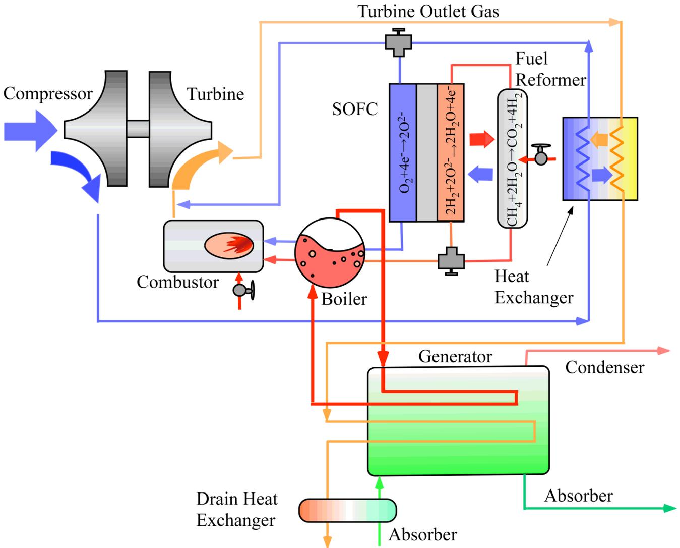
Fig.2 Intermediate wasted heat utilization system
