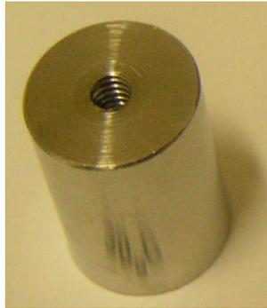
**Figure 4. Polarization Specimen**
